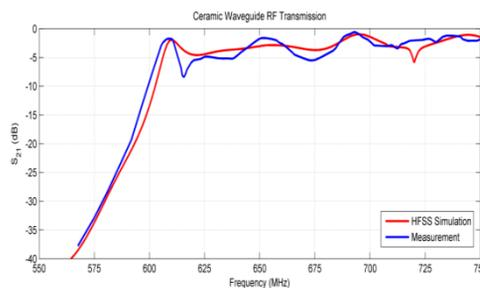
Figure 8: Comparison of the measured transmission across the ceramic waveguide, installed in the eGun vessel, to the transmission simulated in HFSS.
