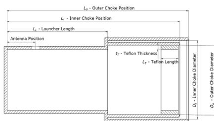
Figure 7: Double-ring choke horn geometry.
