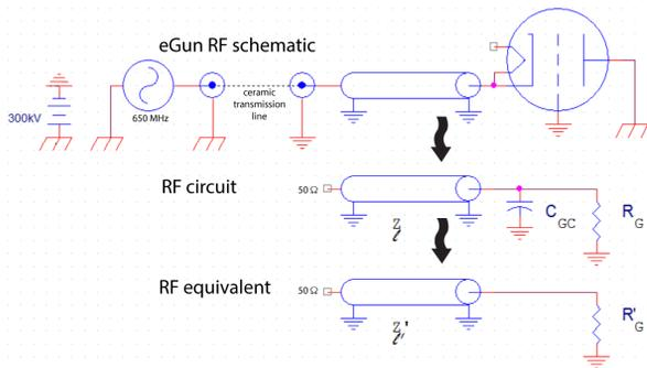
Figure 3: Circuit of the impedance matching section.
