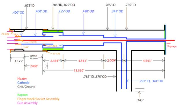
Figure 5: Geometry of the impedance matching section.
