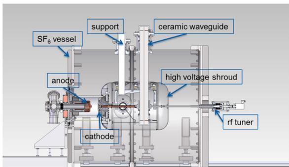
Figure 1: The electron source for the ARIEL eLinac.
