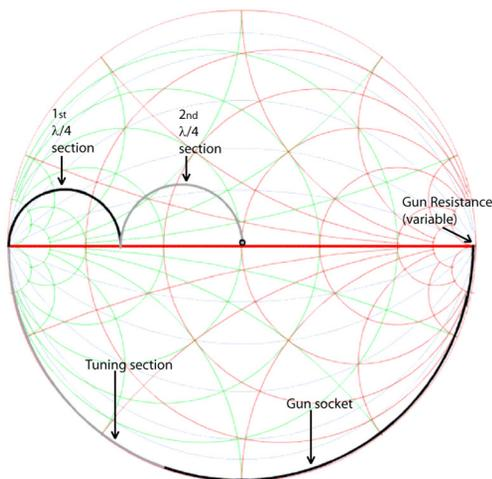
Figure 4: Smith chart of the impedance matching section.
