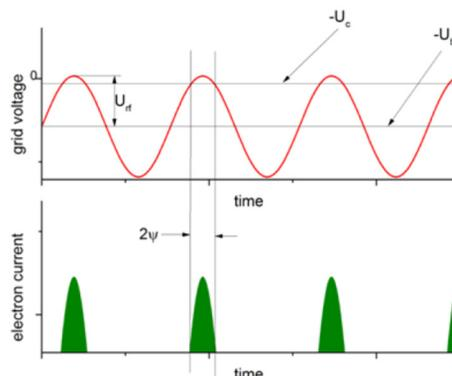
Figure 2: On the top, the time dependant voltage on the cathode grid. When the grid voltage is greater than the cut-off voltage  $-U_c$ , electrons are released, resulting in the electron current shown below.
