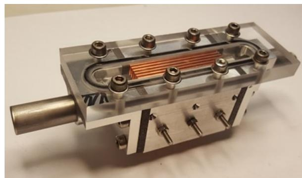
Figure 5: Prototype converter in housing; converter fins are copper surrounded by aluminum housing and a clear polycarbonate lid. Graphite thermally isolates the converter. Heat is applied to the bottom (not visible).
