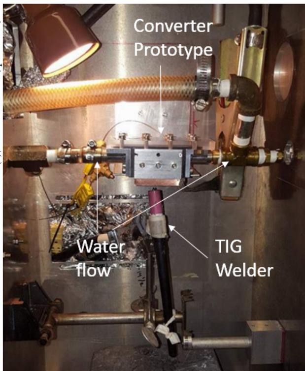
Figure 6: Validation testing apparatus.
