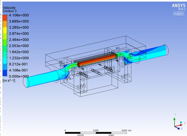
Figure 7: ANSYS CFX Converter Prototype showing flow velocity through the vertical mid plane.
