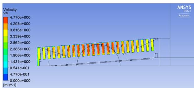
Figure 3: Cross-section through the horizontal plane along the beam axis showing flow balance in water between all fins.
