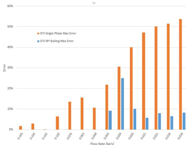
Figure 8: Maximum % difference found between CFX simulations and experimental validation of converter fins with RPI boiling model off and on.
