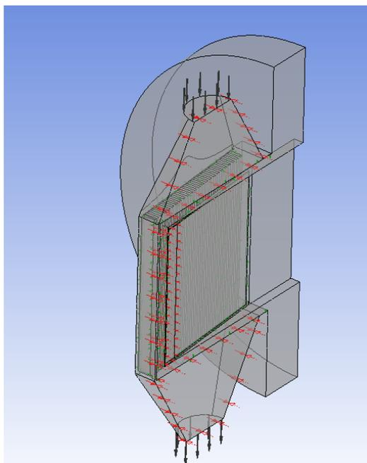
Figure 2: Cross-section through the vertical plane along the beam axis of the converter weldment with diffuser shape designed to evenly distribute flow across all fins. Arrows indicate flow direction.
