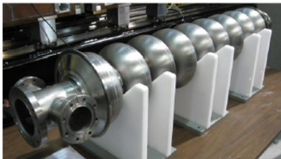
Figure 3: A photo of the unjacketed cavity.
