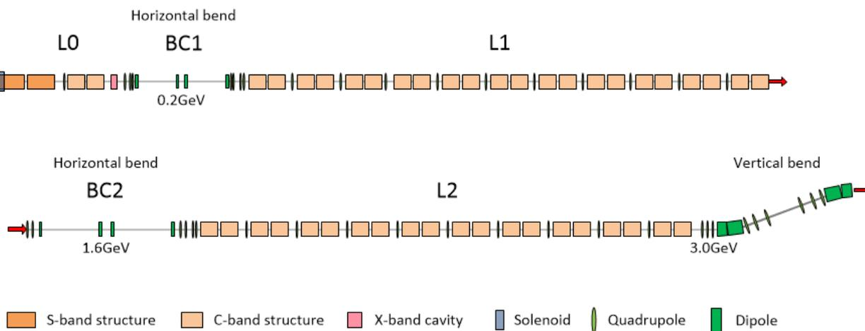
Figure 2: Schematic view of the full-energy linac injector.
