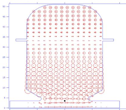
Figure 3: Geometry of the SPS-II TM020 cavity with arrows and circles represent electric and magnetic fields, respectively.
