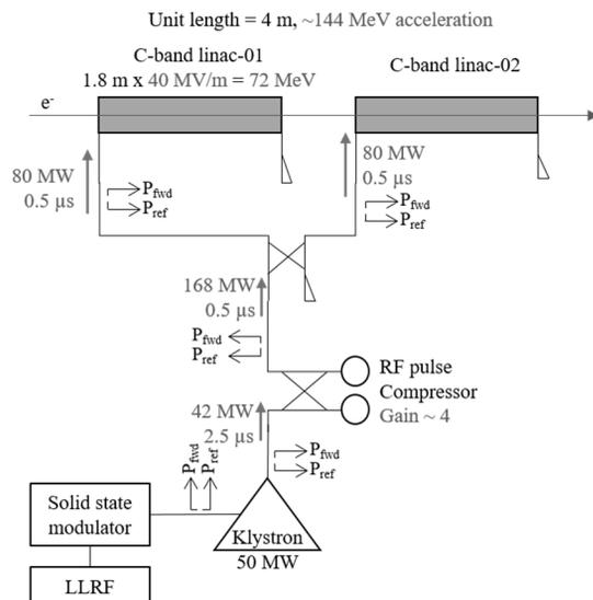
Figure 4: Configuration of the C-band RF unit.
