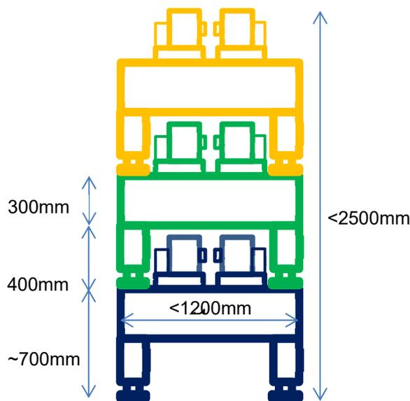
Figure 2: Scheme of stackable horizontal gap undulator.
