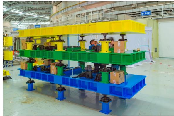
Figure 5: Three frames of stackable horizontal gap undulator.
