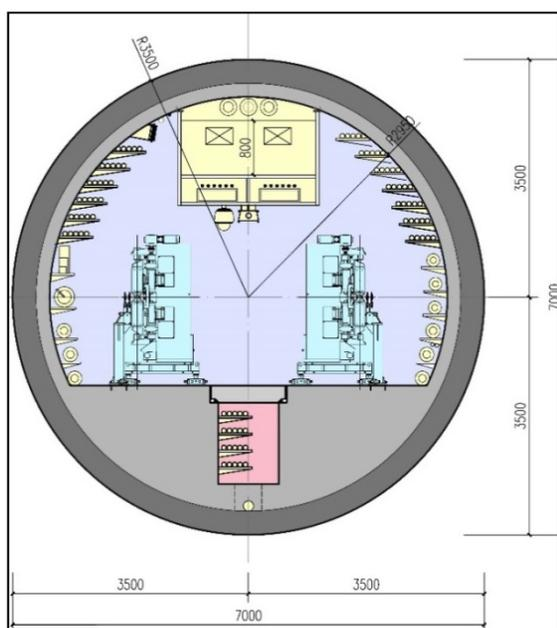
Figure 1: Cross section of undulator tunnel of SCLF.
