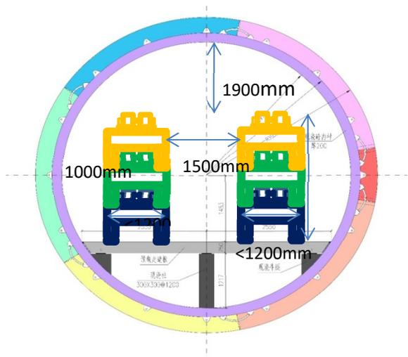
Figure 4: Proposed installations of up to six horizontal gap undulators in the SCLF tunnel with two rows of three-layer layout.
