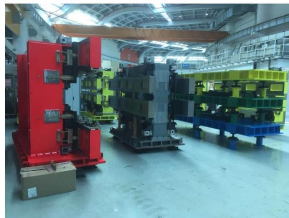
Figure 6: Three kinds of undulator are showing here, red one is a conventional undulator, two-in-one type undulator is in the middle(unpainted) and multi-color stackable undulator frame.
