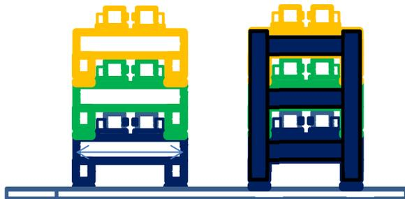
Figure 3: Layout of multi-layer horizontal gap undulators, Left, Stackable type; Right, One-frame type.
