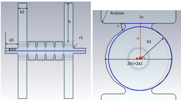
Figure 2: Layout of the racetrack dual-feed coupler. (a) the longitudinal cross section, (b) the transverse cross section.
