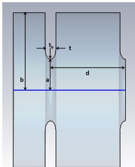
Figure 1: Schematic of the accelerating structure with 1.5 cells.
