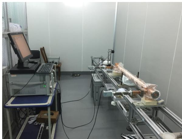
Figure 4: Non-resonant perturbation measurement platform
