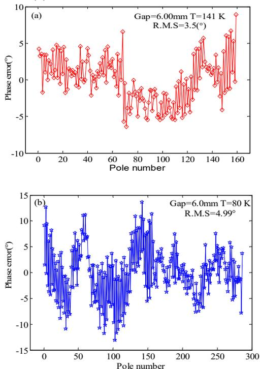
Figure 4: Magnetic field phase error of CPMU (a) CPMU20, (b) CPMU18.
