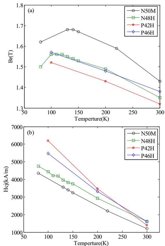
Figure 1: Magnetic properties of magnet for CPMU (a) Remittance, (b) Intrinsic coercivity.
