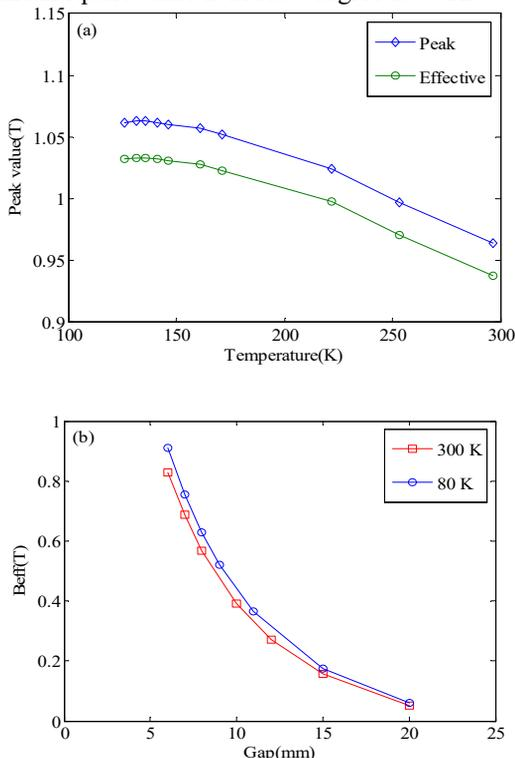
Figure 3: The magnetic field variation of CPMU (a) CPMU20, (b) CPMU18.
