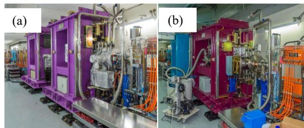
Figure 5: CPMU mounted on storage ring of SSRF (a) CPMU20, (b) CPMU18.
