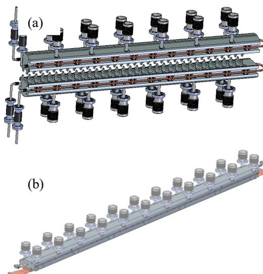
Figure 2: The cooling of the magnet for CPMU (a) CPMU20, (b) CPMU18.
