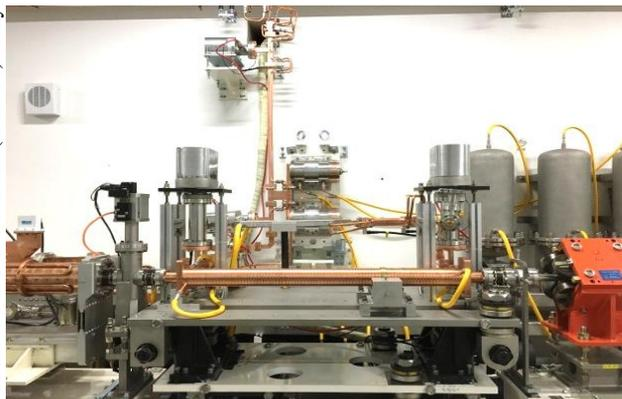
Figure 8: X-band RF unit in SXFEL.
