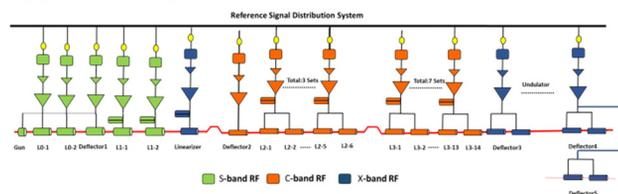
Figure 11: Layout of RF system in SXFEL user facility.
