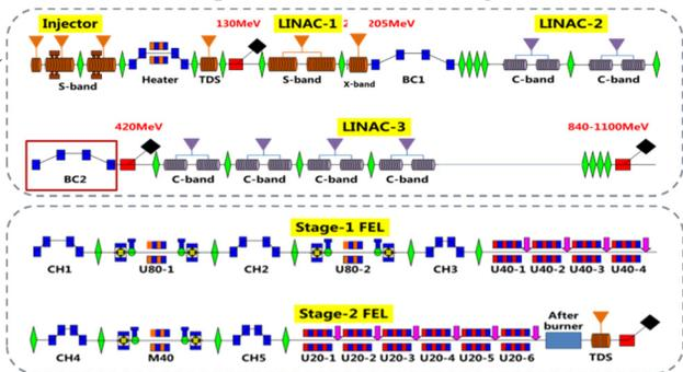
Figure 1: Layout of SXFEL linac (up) and FEL radiation (down).
