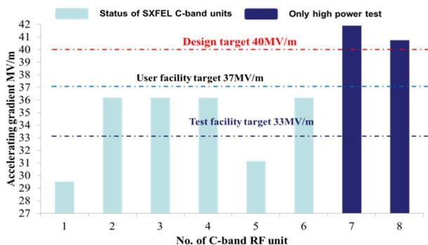
Figure 7: Accelerating gradient of C-band RF units.
