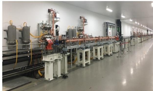
Figure 6: C-band RF acceleration units.
