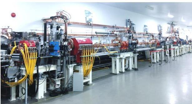
Figure 4: S-band injector and linac-I.
