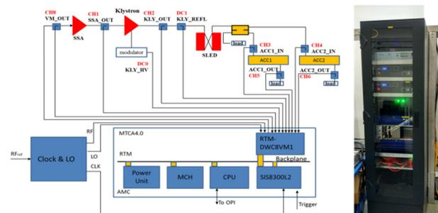
Figure 9: Typical layout of LLRF unit and cabinet.
