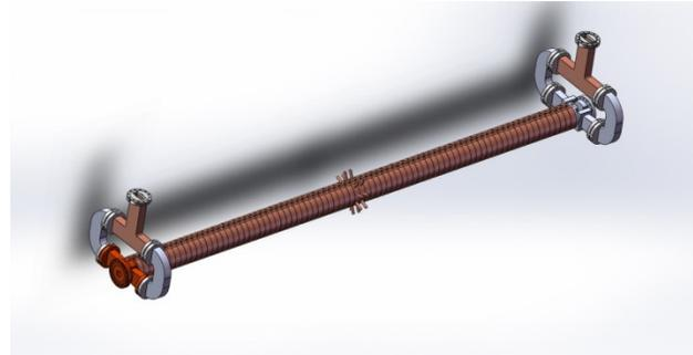
Figure 5: S-band three-meter accelerating structure.
