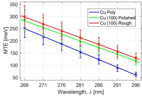
Figure 3: Summary of MTEs as a function of illumination wavelength ( $\lambda$ ) for all photocathode samples.
