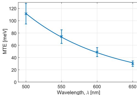
Figure 1: MTE as a function of illumination wavelength for a GaAs photocathode with quantum efficiency around 4%.
