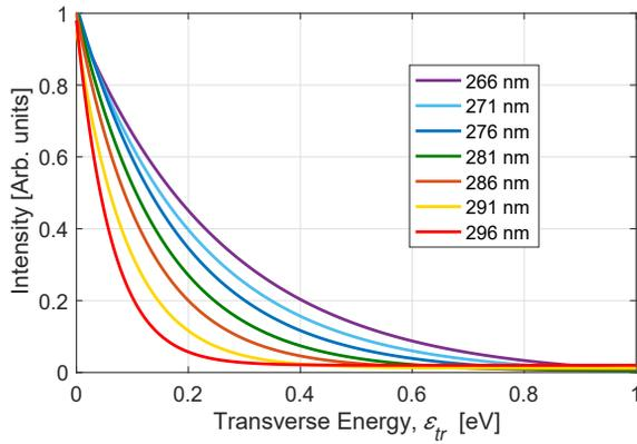
Figure 2: Summary of TEDC fitted curves as a function of illumination wavelength for the Cu.Poly photocathode.
