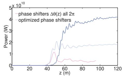
Figure 4: The output peak power as a function of  $z$ . The light-blue and light-red curves are identical to those shown in Fig. 2. The deep-blue curve represents the case with halved undulator segment length.
