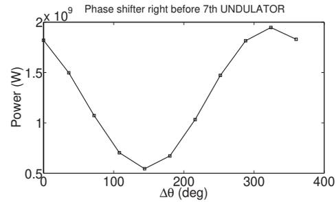
Figure 1: Sinusoidal dependence of the resultant FEL peak power as a function of phase difference between electron beam and the radiation field.
