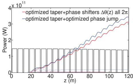
Figure 3: The output peak power as a function of  $z$  for the tapered case. Total taper ratio (7%) is obtained via multidimensional optimization algorithm according to Ref. [6].
