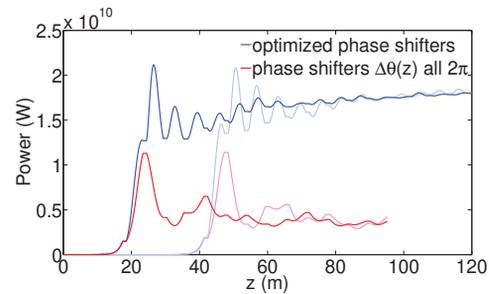
Figure 2: The output peak power as a function of  $z$ . The blue and red curves correspond to the optimized and all- $2\pi$  cases, respectively.
