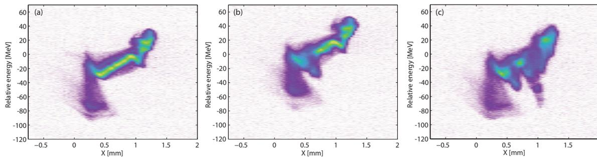
Figure 2: Examples of single-shot electron bunch phase spaces measured downstream of the XTCAV transverse deflection. The horizontal axis corresponds to time, but has been left calibrated in millimeter at the screen because of the horizontal transverse wake effect. (a) lasing off. (b) Two stages amplification. (c) Three stages amplification.
