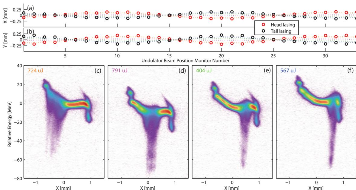
Figure 1: Electron bunch horizontal orbit recorded by the undulator cavity beam position monitors (a). Electron bunch vertical orbit recorded by the undulator cavity beam position monitors (b). The head lasing orbit is represented by red circles and a single shot orange orbit corresponds to the electron bunch phase space in (c). The magenta orbit corresponds to the bunch phase space (d), the green orbit to (e), and the blue orbit to (f).
