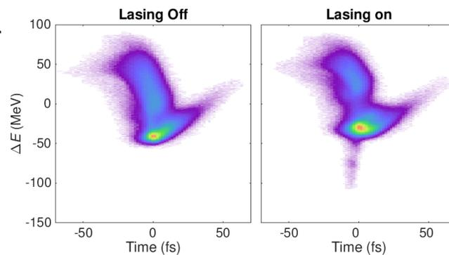
Figure 2: Typical shot of the longitudinal phase space after the undulator showing a lasing suppressed (left) and lasing (right) shot. Note that the size of the lasing shot is artificially increased due to the foil therefore making temporal X-ray reconstruction more difficult. Simulations suggest a pulse length  $< 3$ fs with a measured pulse energy of  $420\mu\text{J}$  with  $7.4$  keV photon energy.
