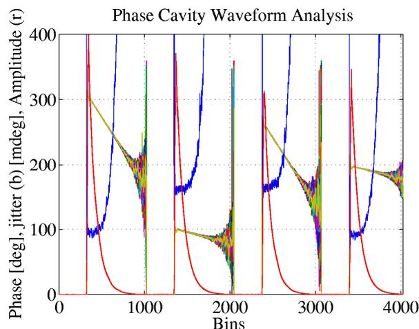
Figure 1: Phase cavity signals with four amplitudes and phases. The two cavities are differently tuned, see slope on 1<sup>st</sup> and 3<sup>rd</sup> signals versus 2<sup>nd</sup> and 4<sup>th</sup>. The phase jitter is lowest on signal 1 and 4 (FEH) while signal 2 and 3 (NEH) is dominated by every-other-pulse (or time slot) jitter.
