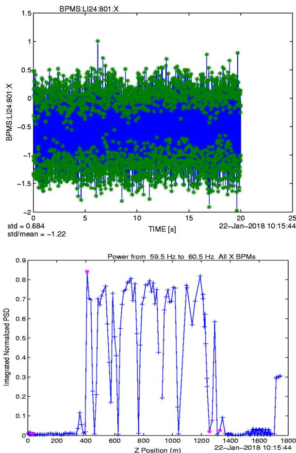
Figure 6: Effect of a -12 MeV time-slot energy offset in BC2 (at 3 MeV) causing a -1.4 mm every other pulse top). Since the leaking dispersion (on purpose to cancel CSR kick) up to 80% of all the jitter downstream is at 60 Hz (bottom). The energy is timeslot corrected at the end of the Linac (Li29/30) so the energy in DL2 (pink dots at  $z = 1300$  m) has no timeslot difference. The transverse difference is corrected by a fast feedback just after DL2.
