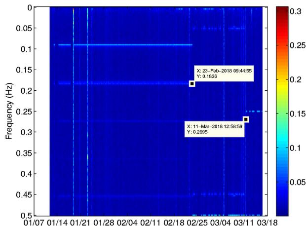
Figure 4: An FFT of the archived fit time revealed exactly when the 11 sec period (0.09 Hz) turns into 2 sec (0.5 Hz), and finally into 4 sec (0.25 Hz).
