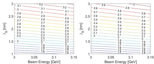
Figure 1: Undulator deflecting parameter  $K$  requirements to satisfy the PAL-XFEL soft X-ray beamline parameters, photon wavelength 1 to 3 nm and electron beam energy 3 to 3.15 GeV, for the cases of 35 mm undulator period (left) and 40 mm period (right).
