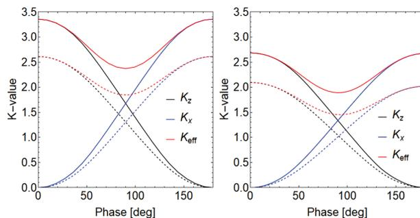
Figure 6: Phase dependence of  $K$  values for the cases of 40 mm (solid lines) and 35 mm (dashed lines) periods in the inclined modes. Two undulator types, APPLE-X (left) and APPLE-II (right), are compared.
