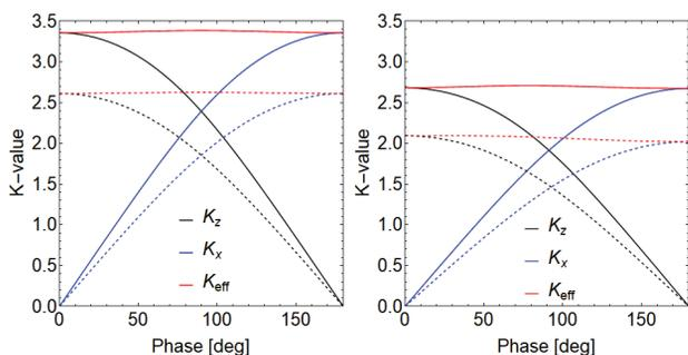
Figure 3: Phase dependence of  $K$  values for the cases of 40 mm (solid lines) and 35 mm (dashed lines) periods in the elliptical modes. Two undulator types, APPLE-X (left) and APPLE-II (right), are compared.
