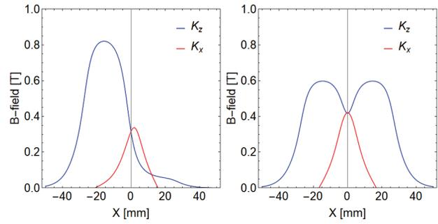
Figure 10: Transverse position dependence of the magnetic field for the energy shift mode (left) and for the gap varying mode (right) of APPLE-II.
