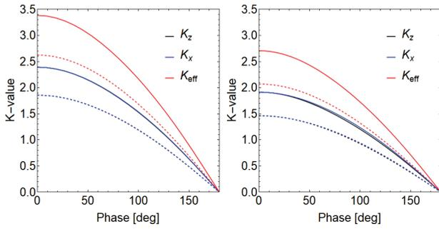
Figure 7: Phase dependence of  $K$  values for the cases of 40 mm (solid lines) and 35 mm (dashed lines) periods in the energy shift modes. Two undulator types, APPLE-X (left) and APPLE-II (right), are compared.
