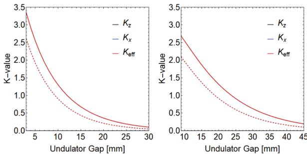
Figure 9: Magnet gap dependence of  $K$  values for the cases of 40 mm (solid lines) and 35 mm (dashed lines) periods in the planar modes. Two undulator types, APPLE-X (left) and APPLE-II (right), are compared.
