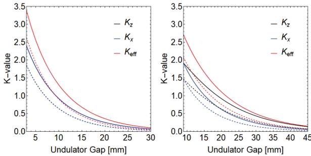
Figure 8: Magnet gap dependence of  $K$  values for the cases of 40 mm (solid lines) and 35 mm (dashed lines) periods in the circular modes. Two undulator types, APPLE-X (left) and APPLE-II (right), are compared.
