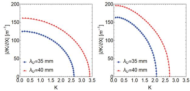
Figure 11: Transverse  $K$  gradient in the energy shift modes of the APPLE-X (left) and APPLE-II (right) types.
