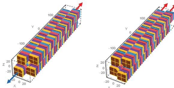
Figure 5: Moving directions of magnet arrays for inclined mode (left) and energy shift mode (right).
