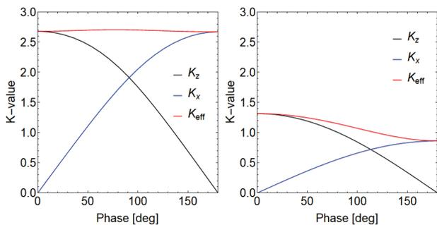
Figure 4: Phase dependence of  $K$  values of the APPLE-II with two different magnet gaps, 9 mm (left) and 20 mm (right), in the elliptical modes.
