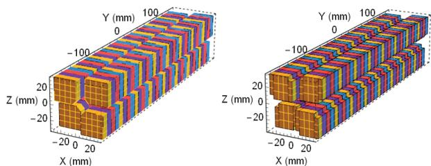
Figure 2: Radia models for APPLE-X (left) and APPLE-II (right) type undulators.
