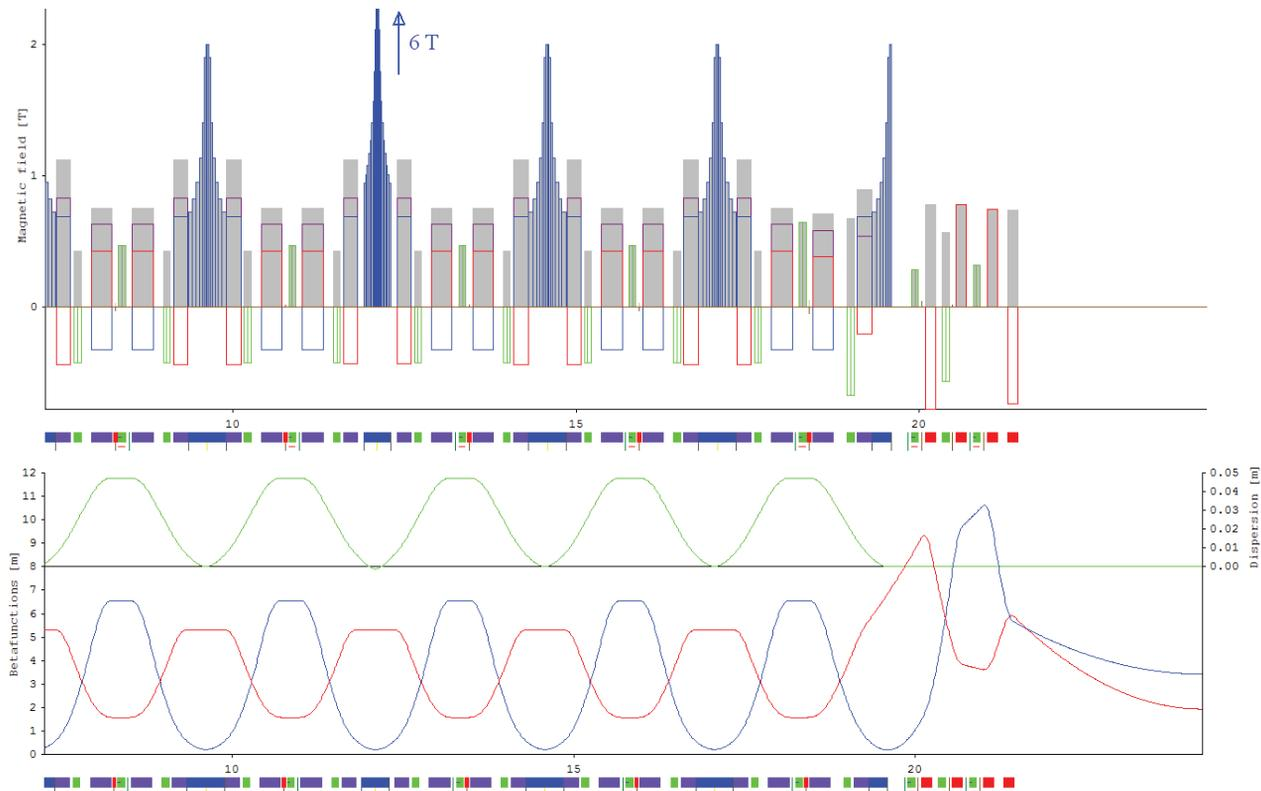
Figure 1: One 7-BA arc (2/3 visible) of the SLS upgrade lattice containing a central super-bend. Top: pole-tip fields for a bore radius of 13 mm (dipole blue, quadrupole red, sextupole green, octupole brown, total as gray bar, and pole-tip field for combined function magnets realized as off-set large aperture quadrupoles in purple). Bottom: optical functions ( $\beta_x$  blue,  $\beta_y$  red, dispersion green).
