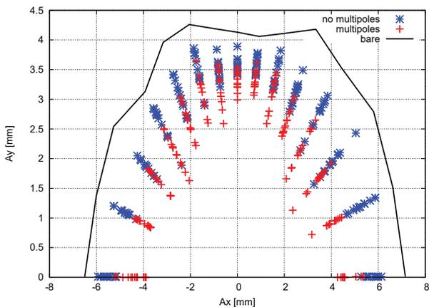
Figure 2: Dynamic aperture for the ideal lattice (solid line) and for 12 seeds of misalignment errors (60  $\mu$ m girder position, 20  $\mu$ m girder to girder, 30  $\mu$ m element to girder, cut 1 sigma) without (blue) and with (red) decapole moments from orbit correctors in sextupoles. The region down to  $x = -5$  mm is required for off-axis injection.
