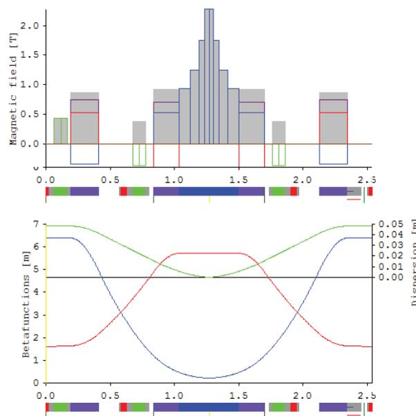
Figure 3: Optics and pole-tip fields for an alternative lattice cell based on high field PM-LGBs and discrete correctors. See caption of Fig. 1 for explanation of plot.
