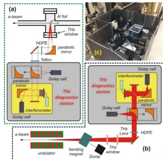
Figure 2: Schematic of the setup of THz measurement for (a) CTR, (b) CUR and THz diagnostics station with the photo shown in (c).
