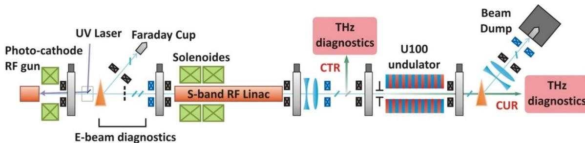
Figure 1: Layout of the NSRRC high brightness photo-injector and coherent THz sources.
