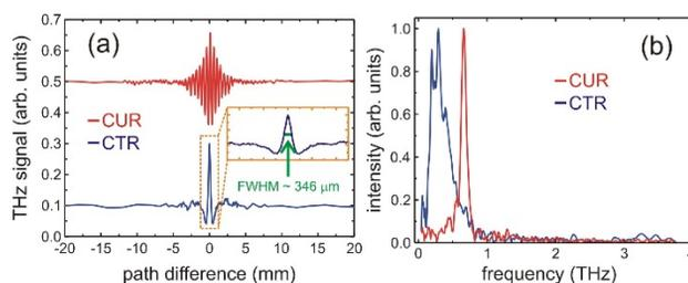
Figure 4: (a) Measured interferograms for CUR (red line) and CTR (blue line) sources. The inset shows the enlargement of the central part of CTR signal. (b) THz spectra retrieved from the interferograms in (a).
