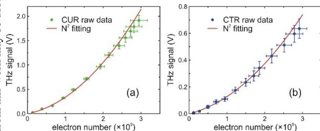
Figure 3: THz output signal as a function of the electron number for (a) CUR and (b) CTR.
