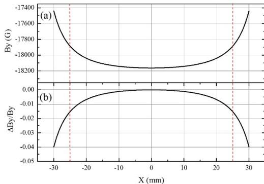
Figure 5: Field distribution (a) and field homogeneity (b) in the transverse direction at the central pole of the W100.
