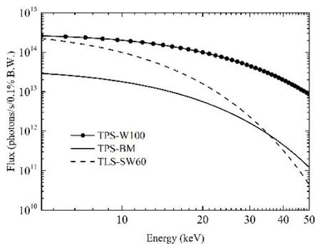
Figure 2: Spectra comparisons for the TPS-W100, TPS-BM and TLS-SW60.
