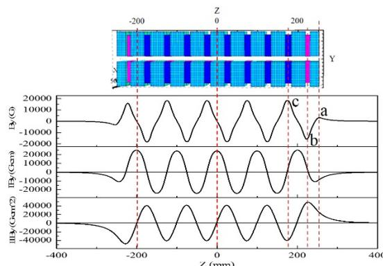
Figure 3: Field distribution for the W100.
