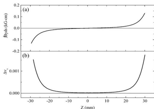
Figure 6: Dynamic field integral (a) and tune shift (b) as a function of the electron beam offset in the W100.
