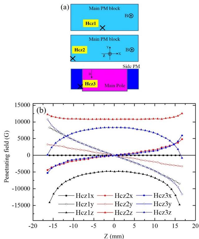
Figure 7: Test points (a) for the penetrating field in the PM block and penetrating field (b) at test points.
