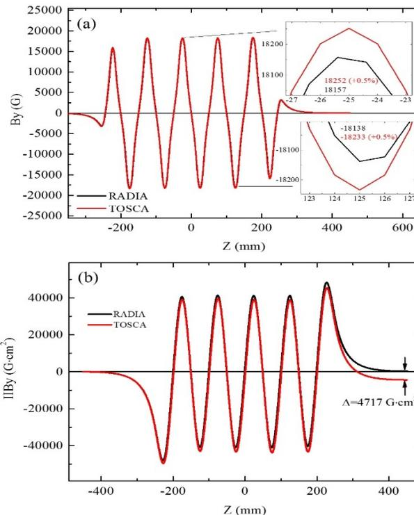
Figure 4: Comparison of the field distribution (a) and electron beam trajectory (b) as calculated by RADIA and TOSCA.
