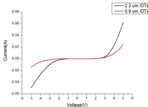
Figure 7: I-V for  $2.3\text{ }\mu\text{m}$  and  $0.9\text{ }\mu\text{m}$  IDTs SAW devices.
