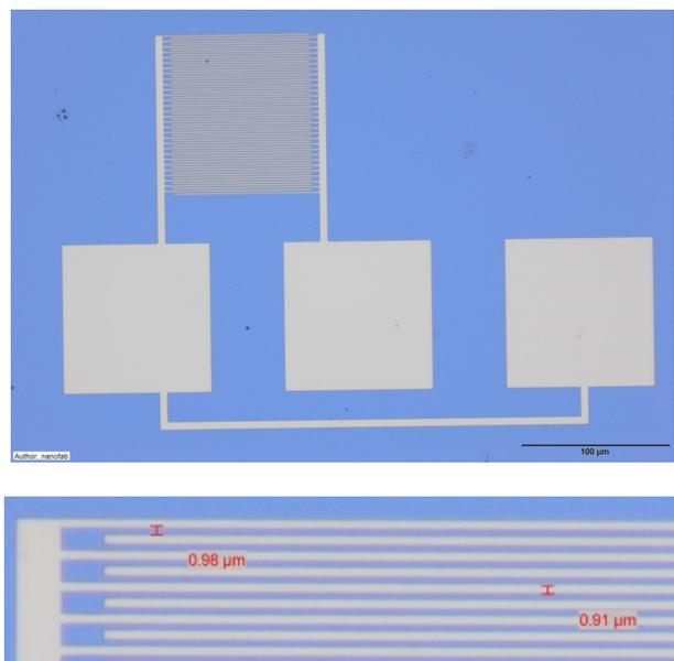
Figure 6: Structure of metal IDTs (0.9um).
