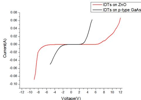
Figure 8: I-V SAWs devices with and without ZnO.
