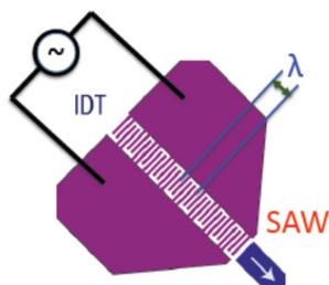
Figure 1: Schematic layout of SAW generation.
