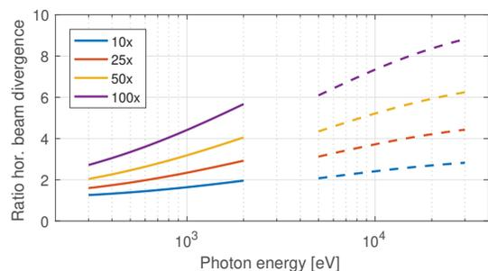
Figure 4: Ratio between horizontal photon beam divergence for excited and unexcited bunch as function of photon energy and 10, 25, 50 and 100 times emittance increase. Two typical examples for soft (solid) and hard (dashed) X-ray beamlines are displayed.
