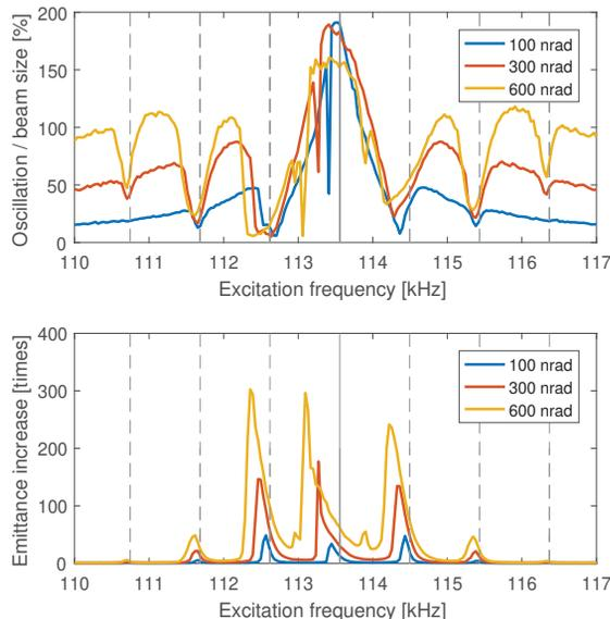
Figure 2: Ratio between simulated beam oscillation and beam size (top) and emittance increase (bottom) as function of horizontal excitation frequency for the design optics for different kick amplitudes. The position of the betatron tune (solid) and the synchrotron sidebands (dashed) are marked.
