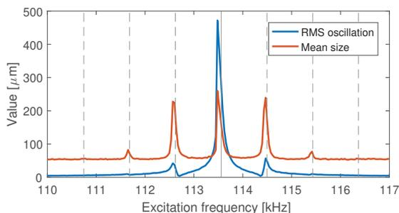
Figure 1: Simulation of beam oscillation (RMS) and size as function of horizontal excitation frequency for the design optics with a 50 nrad kick. The position of the betatron tune (solid) and the synchrotron sidebands (dashed) are marked.
