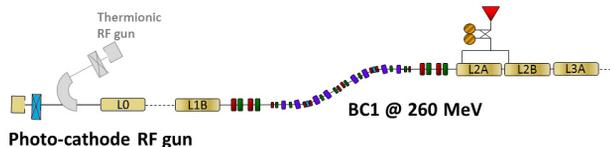
Figure 1: Overview of the MAX IV injector where the photo-cathode gun is to the lower left. It is followed by a solenoid and then the first linac structure (L0). BC1 is the first bunch compressor after 3 linac structures at an energy of 260 MeV, and is followed by the main linac.
