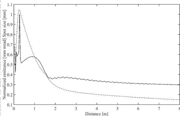
Figure 5: Evolution of the projected emittance for the full two beam (solid) and for the spot size (dashed).
