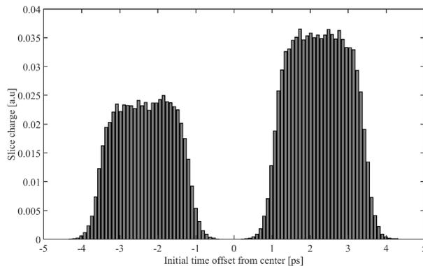
Figure 2: Initial longitudinal bunch distribution for the driver-witness acceleration.
