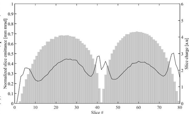
Figure 4: Slice emittance and charge distribution for the driver-witness beam at the end of the first linac (approximately 7 m).
