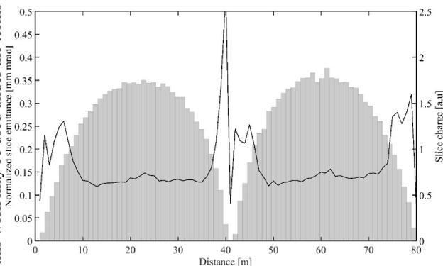
Figure 6: Slice emittance and charge distribution of the two color beam at the end of the first linac (approximately 7 m).
