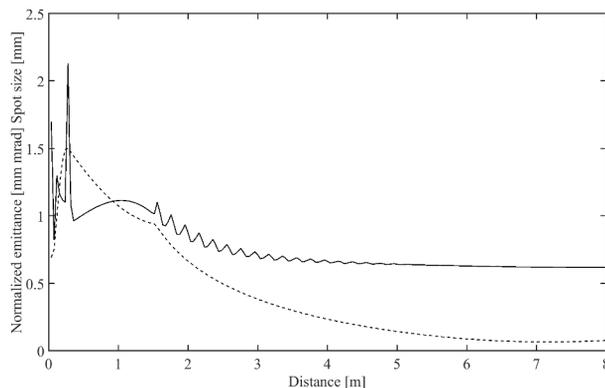
Figure 3: Evolution of the projected emittance for the full beam (solid) and for the spot size (dashed).
