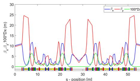
Figure 1: Optical functions and lattice structure for one cell of the HEPS storage ring.
