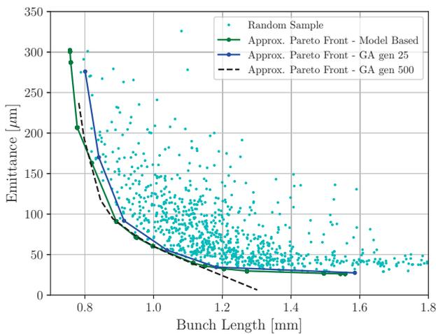
Figure 3: Comparison of model based optimization and the GA implemented in OPAL at 40 nC.
