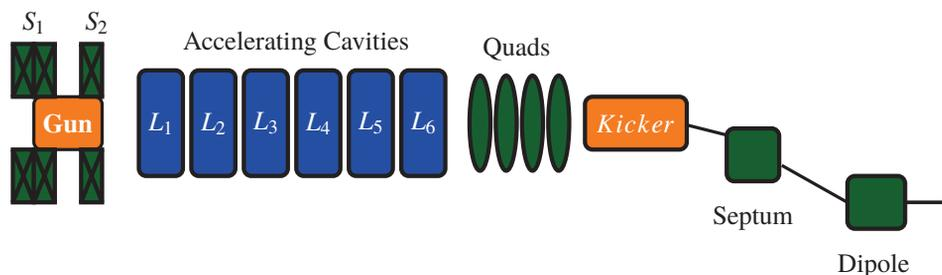
Figure 1: Partial beam line layout at the AWA.
