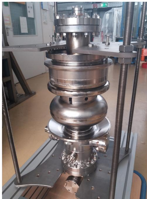
Figure 1: Gun 1.1, mounted in a frame for vertical testing. Beam pipe side downwards, full cell in the picture's center, half cell above. The choke cell is hidden in the cylindrical housing in the upper part.
