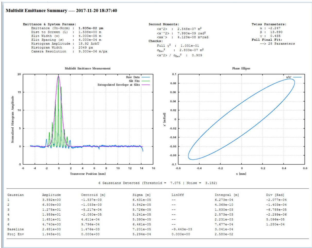
Figure 2: An example of the multi-slit Python measurement routine output, generated with each call of the routine. Final beam parameters are displayed on the top while the histogram of the slit image is shown in the left with fitted peak and fitted beam envelop information at the slit location. The phase ellipse is displayed on the right side.
