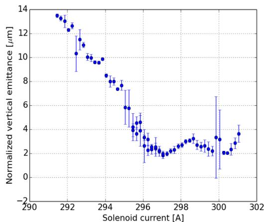
Figure 3: Emittance at 250pC vs gun solenoid scan data. All data shown was collected real time and re-evaluated offline. During this scan main and bucking solenoid is kept in a fixed ratio to minimize magnetic field at the photocathode.
