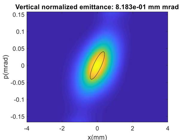
Figure 4: Phase diagram from a one-shot multi-slit measurement for 100pC beam. The black circle is drawn from Twiss parameters calculated in the measurement. The intensity map was drawn with interpolation of the measured data.
