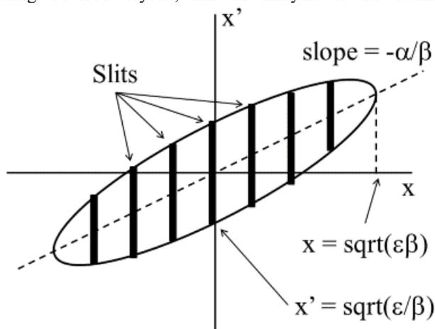
Figure 1: Diagram showing parametrization of phase space ellipse relevant to multi-slit technique.
