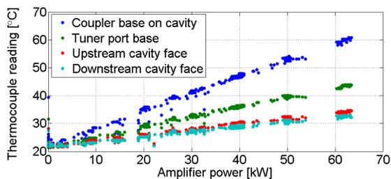
Figure 3: Temperatures recorded during conditioning.
