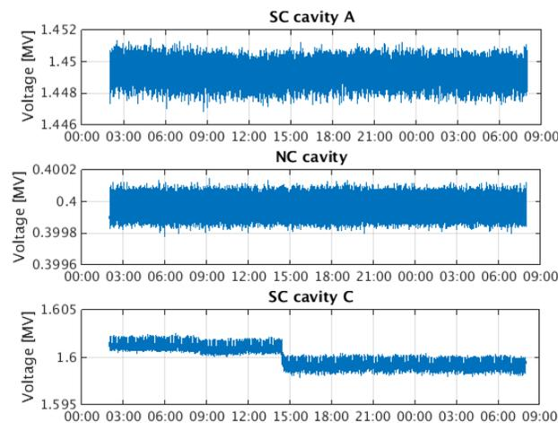
Figure 9: Long-term stability of cavity voltages.
