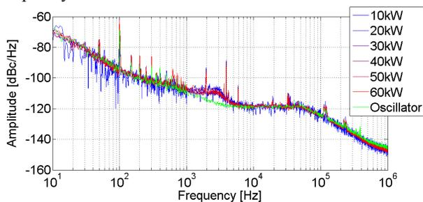
Figure 4: Phase noise at cavity pick-up.
