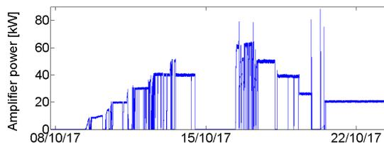
Figure 2: Cavity conditioning record.
