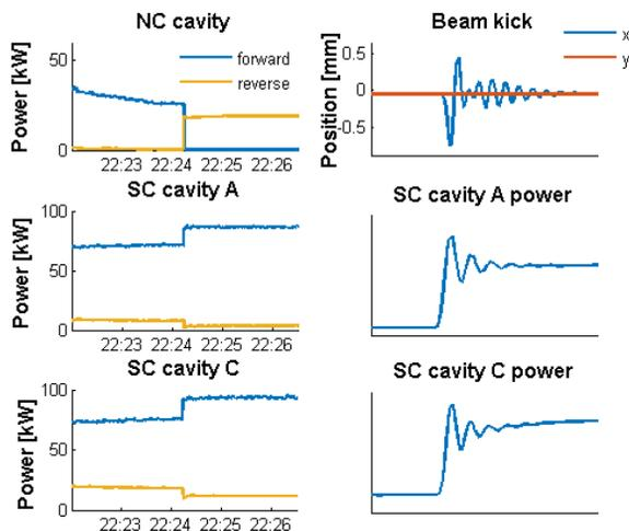
Figure 8: Response to the loss of NC cavity power.
