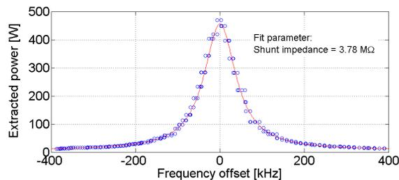
Figure 6: Cavity detuning with a 20 mA beam.
