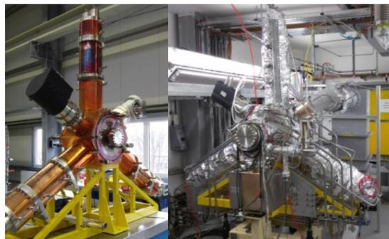
Figure 1: Cavity delivered by the manufacturer (left) and prepared for operation by DLS (right).
