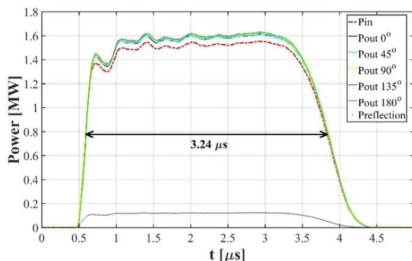
Figure 7: High-power test results of the rotary joint.
