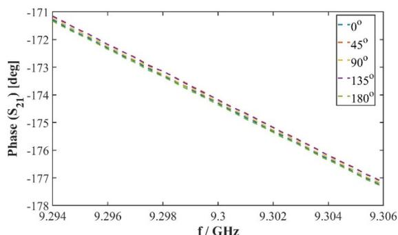
Figure 4: Measured results of phase drift with the different rotation angles after brazing.
