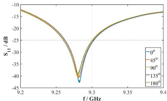
Figure 3: Measured results of reflection with the different rotation angles after brazing.
