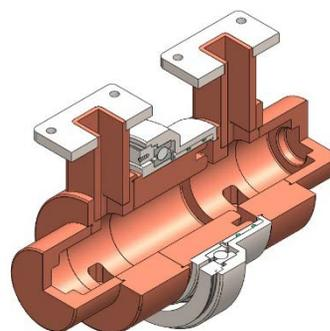
Figure 2: Mechanical design of the rotary joint.
