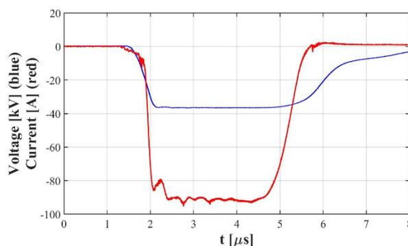
Figure 6: Waveforms of the magnetron voltage and current.
