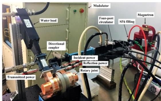
Figure 5: Setup of the high-power test of the rotary joint.
