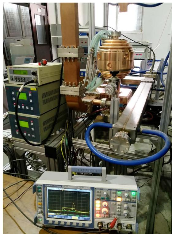
Figure 11: The pulse compressor under high power test.
