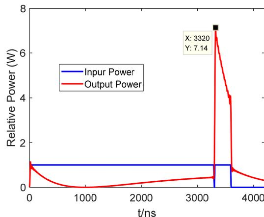
Figure 1: Input and output waveforms of the pulse compressor with compression ratio of 12.
