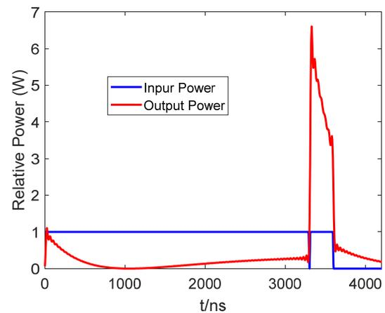
Figure 7: Input and output powers of the pulse compressor after brazing.
