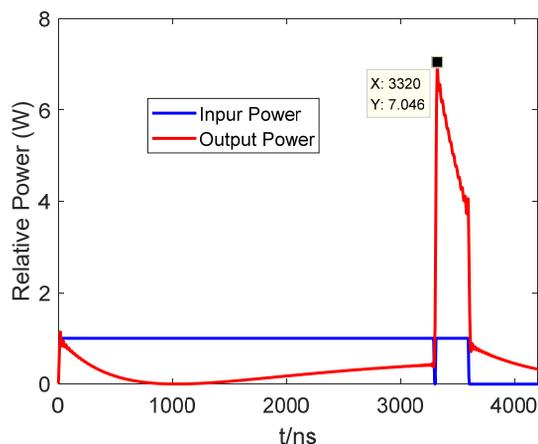
Figure 10: Input and output powers of the pulse compressor after the tuning.
