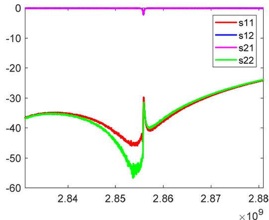
Figure 9: S-parameters of the pulse compressors after the tuning.
