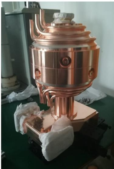
Figure 4: Pulse compressor after brazing.
