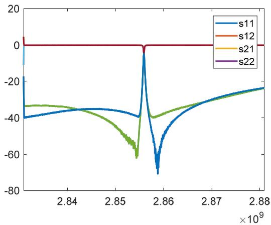
Figure 5: S-parameters of the pulse compressor after brazing.
