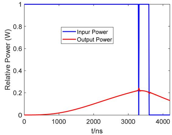
Figure 6: Input and reflected powers of the pulse compressor after brazing.
