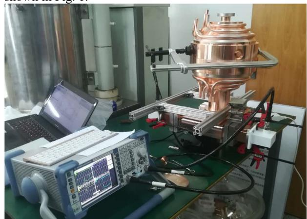
Figure 8: Tuning of the pulse compressor.
