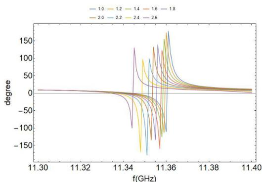
Figure 6: The phase curves of the cavity model with different values of the relative permeability.
