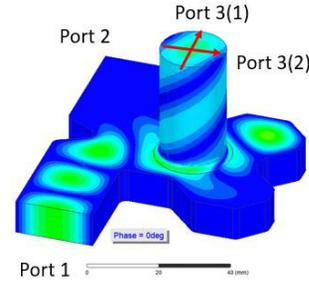
Figure 2: The simulation model of the revised RF polarizer.
