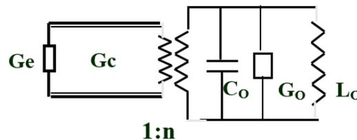
Figure 1: The equivalent circuit of a resonant cavity coupled with a transmission system.
