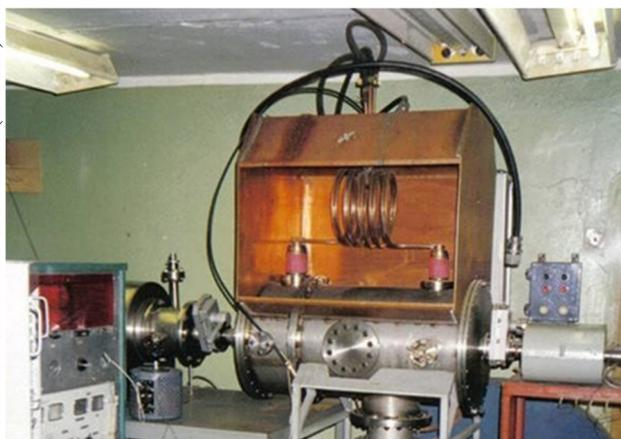
Figure 1: The 250 keV Implanter of single charged nitrogen ions.
