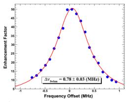
Figure 4: Frequency tuning curve of DREC at various frequencies applied to acousto-optic frequency shifter (AOFS). Dots are the experimental data, and red curve is the calculated results from the theoretical model.
