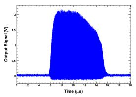
Figure 3: Typical macropulse waveform of the transmitted UV beam when the cavity is locked in a double resonance frequency setting with a constant frequency shift.
