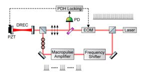
Figure 1: Locking principle of doubly-resonant enhancement cavity (DREC) operating with burst-mode laser pulses.
