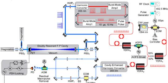
Figure 2: Experimental setup of burst-mode Fabry-Perot cavity for ultraviolet pulse enhancement in a double-resonance configuration. PBS, polarization beam splitter; QWP, quarter-wave plate; HWP, half-wave plate; PZT, piezoelectric g quency shifter; YDFA, ytterbium doped fiber amplifier; PDH, Pound-Drever-Hall.
