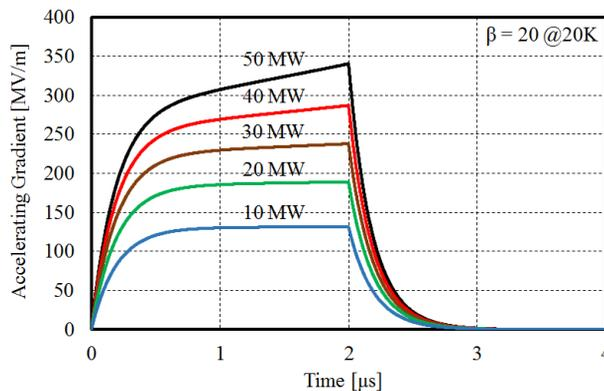
Figure 2: The accelerating gradient obtained with the cold model cavity for each input power.
