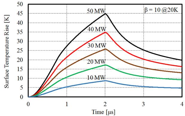
Figure 7: Average surface temperature rise when each input rf power was modulated as shown in Fig. 5.
