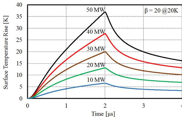
Figure 3: Average surface temperature rise in the cold model cavity for each input power.
