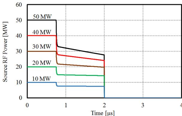
Figure 5: The waveforms of the input rf power modulated by the function in Eq. (6). The parameters  $a$  and  $b$  were optimized for each input rf power.
