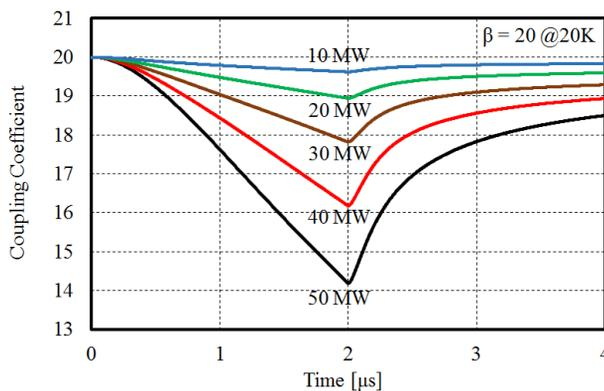
Figure 4: Decrease in the coupling coefficient due to the surface temperature rise.
