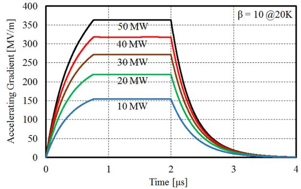
Figure 6: The flat accelerating gradient obtained with the input rf power modulation for each input power.
