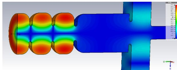
Figure 1: Magnetic field distribution in the cold model cavity by the CST Studio simulation [5].
