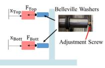
Figure 5: Tuner test stand setup, this shows the location of Belleville washers and where the displacement measurements take place.
