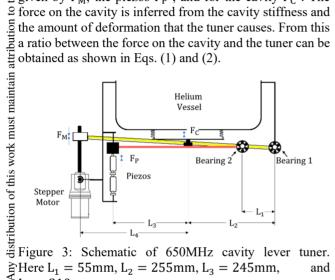
Here  $L_1 = 55$ mm,  $L_2 = 255$ mm,  $L_3 = 245$ mm,  $L_4 = 310 \text{mm}.$
