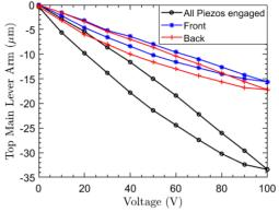
Figure 8: Top main lever arm displacement with the respect to the piezo voltage.
