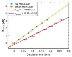
Figure 6: Force generated by adjustment screw and displacement in the main top and bottom lever arms.
