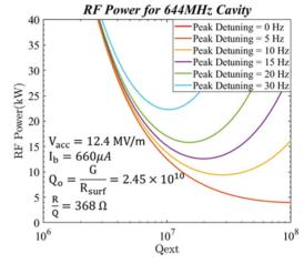
Figure 1: As the peak detuning goes up so does the RF power. Parameters are based on the FRIB cavity [4].
