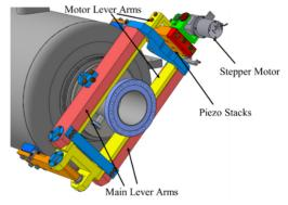
Figure 2: The jacketed 644MHz cavity with the tuner attached.
