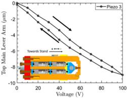
Figure 7: Configuration of the piezo encapsulations is shown. The displacement caused by piezo number 3.
