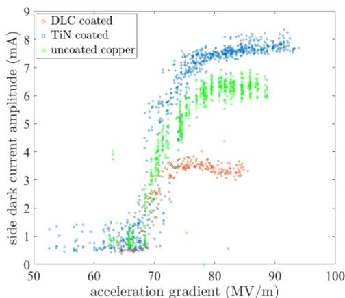
Figure 8: Side dark current amplitude measured at different acceleration gradient levels.
