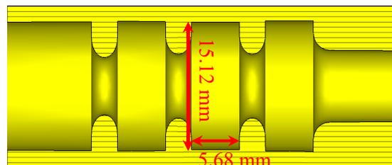
Figure 1: Axisymmetric view of the 17 GHz MIT-DLWG structure.
