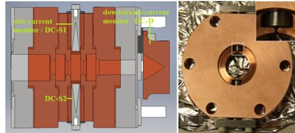
Figure 5: Accelerator structure for high power testing (left). Two Faraday cups, DC-S1/S2, measure the side dark currents, and another current monitor, DC-D, measures the downstream dark current; the thin slits on the side wall of the fabricated part (right).
