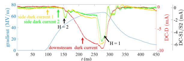
Figure 6: Sample traces of the structure acceleration gradient, downstream dark current and side dark currents. The high power microwave pulse is a square pulse with a pulse length of 210 ns.
