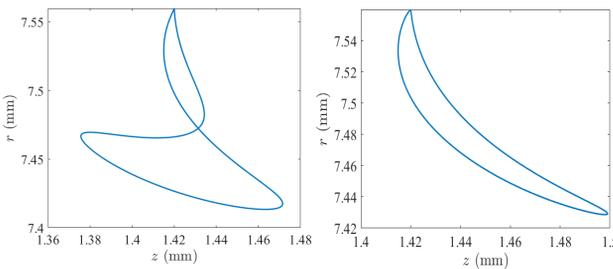
Figure 4: Multipactor trajectories for the  $H = 2$  mode (left) at an acceleration gradient of 45 MV/m and the  $H = 1$  mode (right) at 72 MV/m. In both trajectories, the electron is released at  $z_0 = 1.42$  mm with an initial energy of 2 eV. Side wall is located at  $r = 7.56$  mm.
