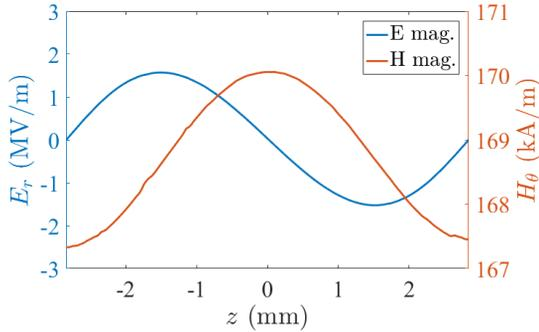
Figure 2: The axial distribution of the radial electric field magnitude and azimuthal magnetic field magnitude on the central cell side wall for an acceleration gradient of 45 MV/m (simulation in CST Microwave Studio [4]).
