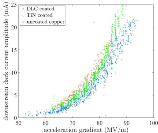
Figure 7: Downstream dark current amplitude measured at different acceleration gradient levels for the structures with different central cell side wall surface conditions.
