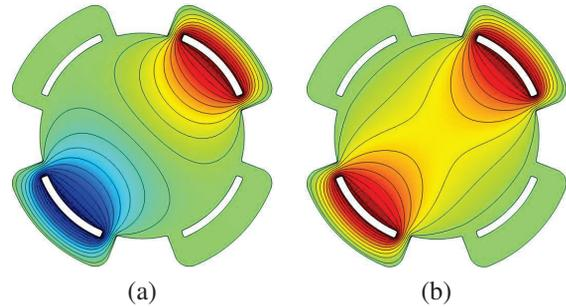
Figure 1: The electric scalar potential over a stripline cross-section obtained numerically in COMSOL Multiphysics [8] for the odd (a) and even (b) TEM mode. The odd and even modes are excited when applying transverse and longitudinal feedback, respectively.
