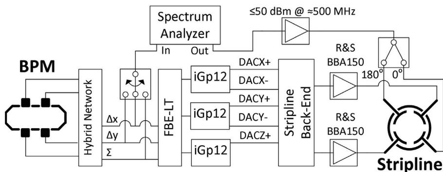
Figure 3: The set-up of the BBB feedback system.
