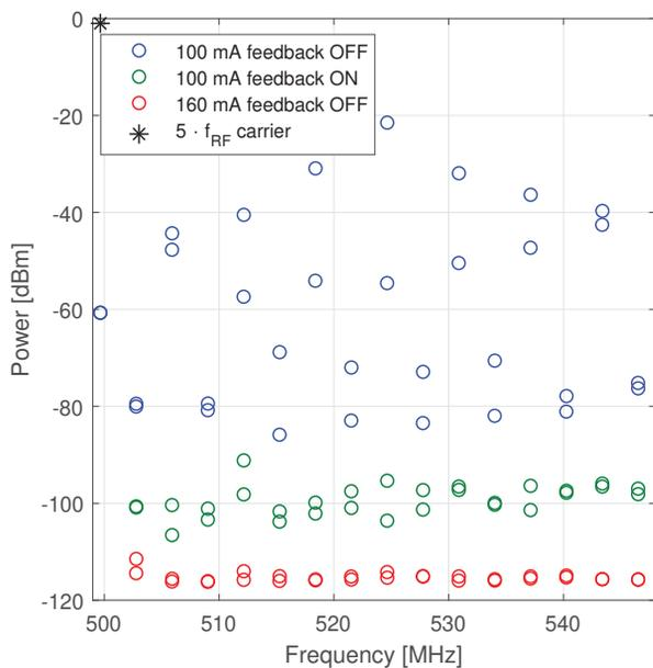
Figure 5: The magnitude of all the 32 coupled bunch modes obtained from the BPM sum signal. The measurement is done with a spectrum analyzer at different beam currents.
