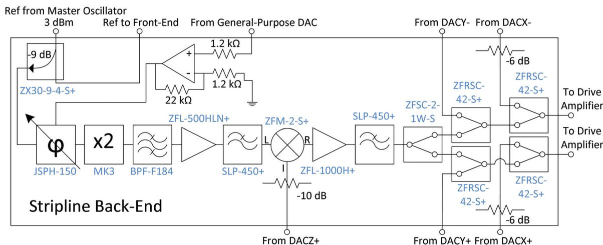
Figure 4: The circuit diagram of the stripline back-end. All part numbers (in blue) are from the Mini-Circuits' catalogue.
