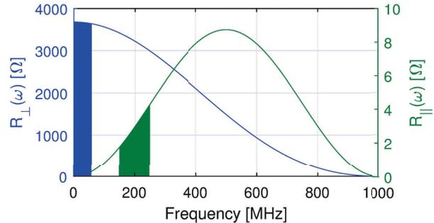
Figure 2:  $R_{\perp}(\omega)$  and  $R_{\parallel}(\omega)$  obtained from (1) and (2), respectively. The blue and green areas show the frequency spans where the transverse and longitudinal feedback are applied, respectively.
