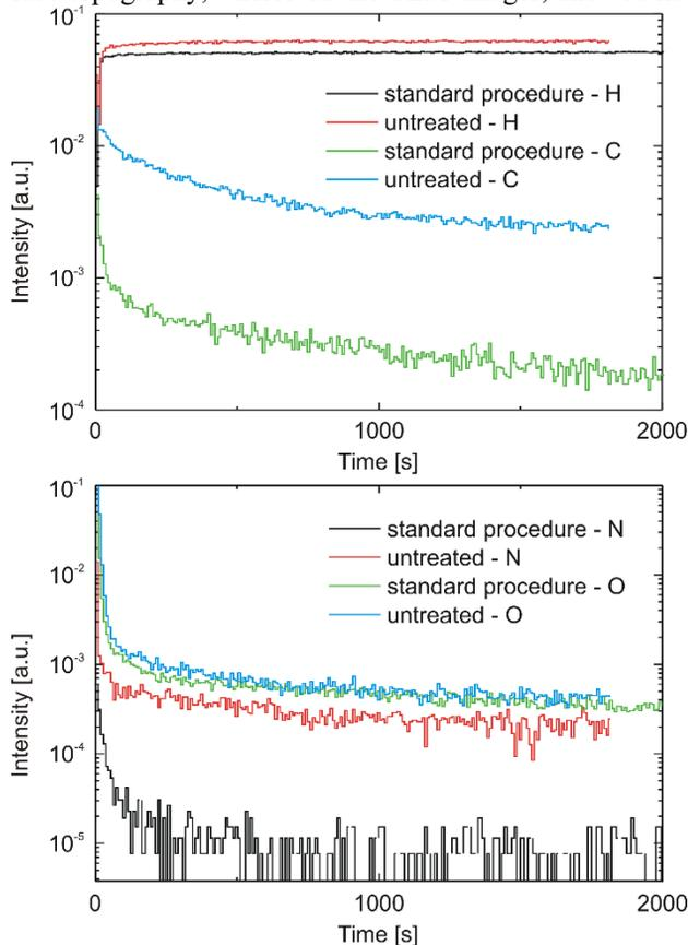
Figure 3: SIMS depth profiles for the elements H, C, N, and O for standard-processed and for untreated samples.
