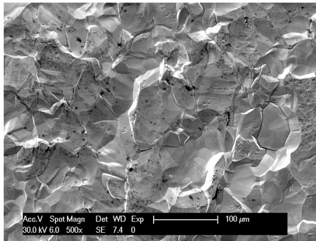
Figure 2: SEM image of an untreated Niobium sample.
