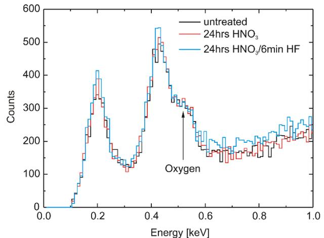
Figure 5: Comparison of the low-energy EDX spectra of three different niobium samples.
