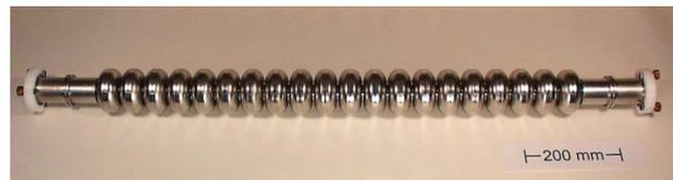
Figure 1: 3 GHz 20-cell Niobium cavity.
