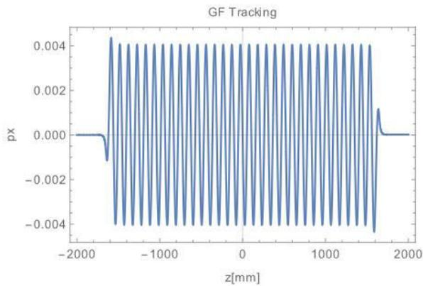
Figure 5: Normalized momentum trajectory of horizontal direction of 800-MeV electron with 2<sup>nd</sup> order GF tracking method
