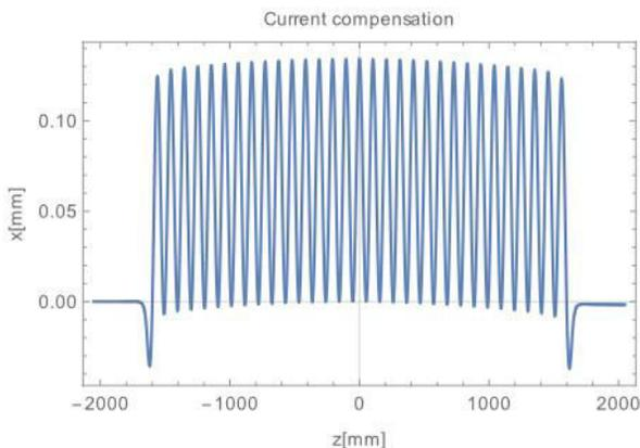
Figure 6: Normalized trajectory of horizontal direction of 800-MeV electron after current compensation.
