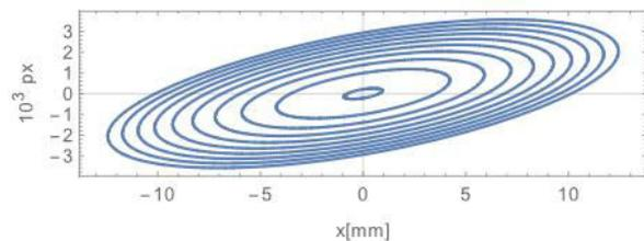
Figure 8: Normal form analysis of the whole ring after current compensation.
