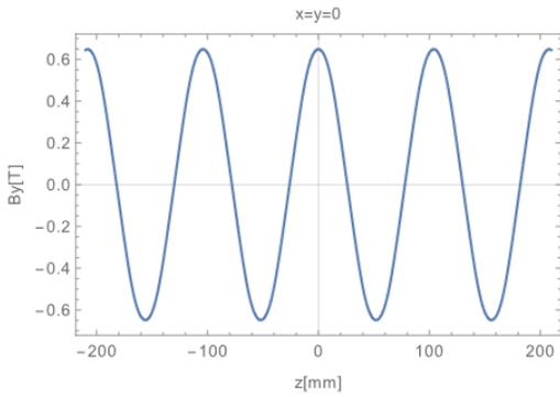
Figure 1: On-axis vertical magnetic field distribution along longitudinal direction (4 periods) in horizontal polarization mode.
