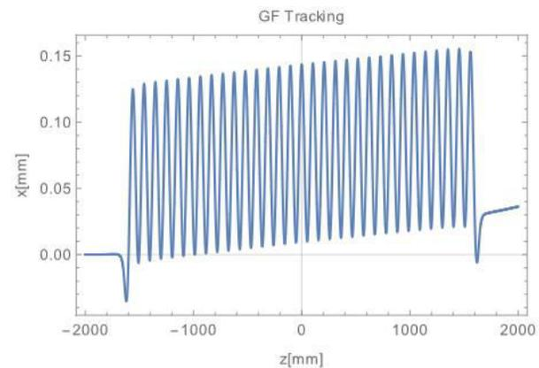
Figure 4: Trajectory of horizontal direction of 800-MeV electron with 2<sup>nd</sup> order GF tracking method.
