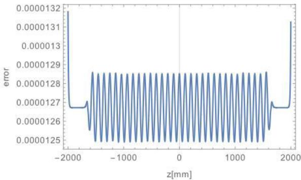
Figure 3: Errors of vertical magnetic field obtained by surface fitting method and Fourier expansion model.
