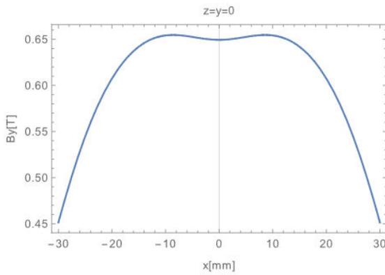
Figure 2: On-axis vertical magnetic field distribution along horizontal direction in horizontal polarization mode.
