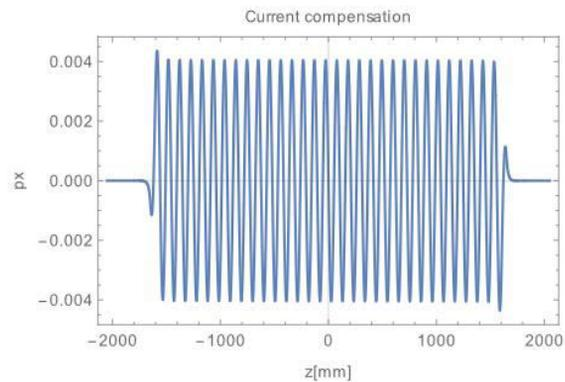
Figure 7: Normalized momentum trajectory of horizontal direction of 800-MeV electron after current compensation.
