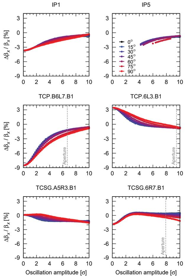
Figure 3: Horizontal amplitude-dependent  $\beta$ -beating at the interaction points of the HL-LHC baseline, and at selected primary (TCP) and secondary (TCSG) collimators, at the start of the fill.
