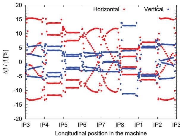
Figure 1: Horizontal and vertical  $\beta$ -beating at zero amplitude along the machine for the HL-LHC baseline at the start of the fill.
