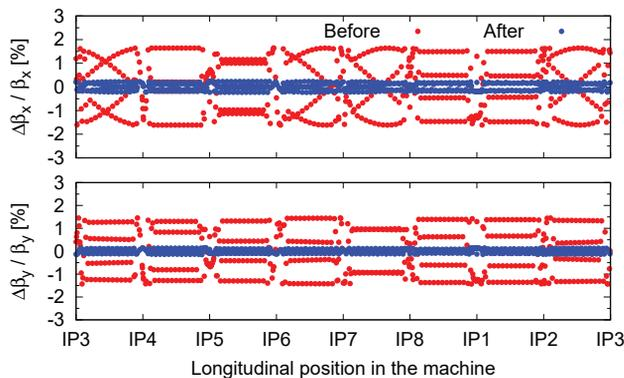
Figure 4: Horizontal and vertical  $\beta$ -beating before and after correction of the quadrupolar term of the BBLR with a sextupole magnet with offset.
