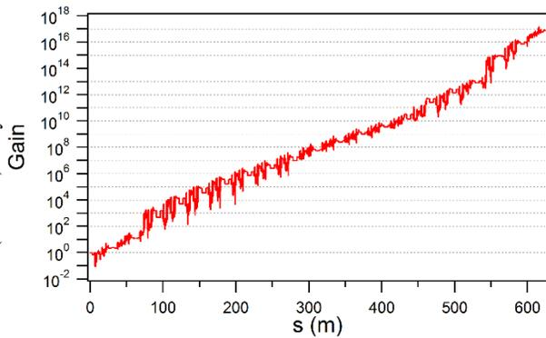
Figure 3: Even an arc with a modest gain (1.5) will lead to unacceptably large microbunching gain over many turns.
