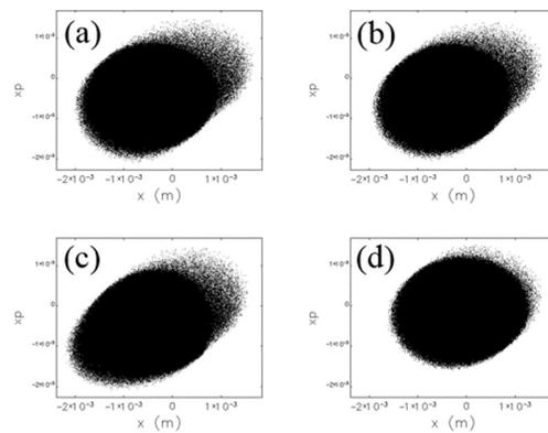
Figure 5: Horizontal phase space at the exit of the simple arc simulating CSR with (a) elegant (b) GPT (c) GPT including space charge (d) Bmad including the effects of shielding from a 2" full aperture.
