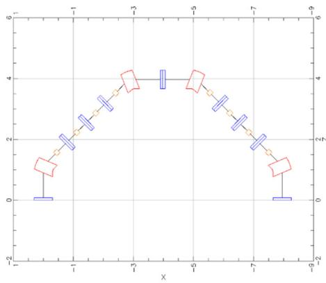
Figure 2: Floor plan of a simple isochronous arc. Red markers denote dipoles, blue markers denote quadrupoles and orange markers denote sextupoles.
