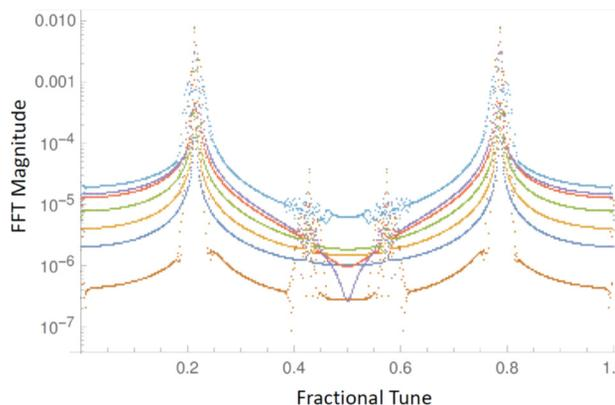
Figure 9: The FFT at 70% of bucket height of the redesigned booster with varied momentum offsets, showing the absence of synchrotron coupling.
