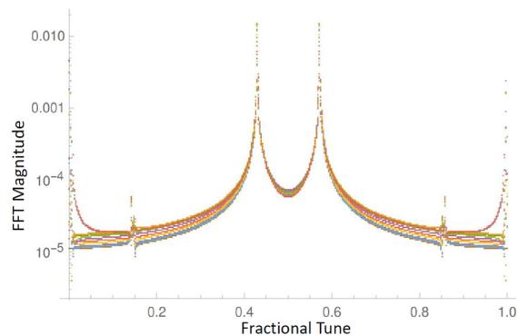
Figure 3: FFT of the horizontal motion of various momentum offsets at injection in the ring, showing synchrotron coupling at edges of the plot.
