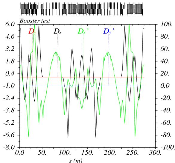
Figure 2: Linear and nonlinear dispersions in the lattice of the previous booster design [2].
