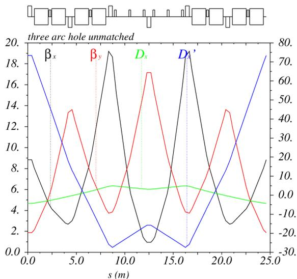
Figure 4: This is the base FMC cell being used in the revised booster. Sextupoles between the dipoles, and at their equivalent positions in the empty areas are used to control the nonlinear dispersions in the ring, the other sextupoles are present for chromaticity correction.
