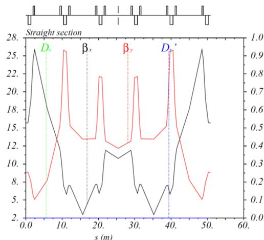
Figure 6: This is one of the straight sections of the machine, this section contains the RF accelerating cavity.
