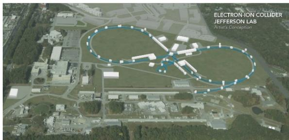
Figure 1: This is a layout of the proposed JLEIC footprint on the Jefferson Lab site. The small figure-8 shape is the booster described here.
