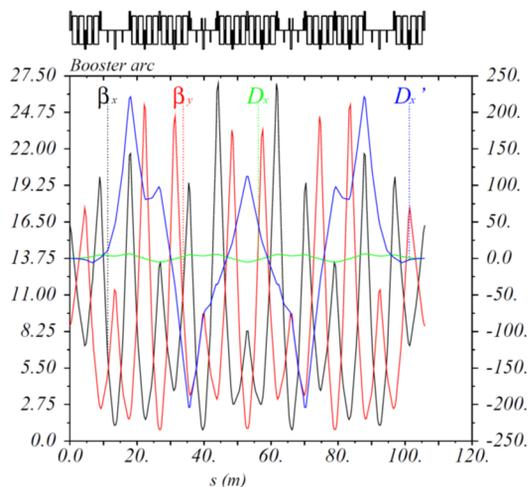
Figure 5: One of the arcs in the booster, the nonlinear dispersions are corrected such that they are zero in the straights.
