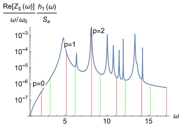
Figure 6: Summand of effective impedance for two different coupled-bunch modes (electron ring).
