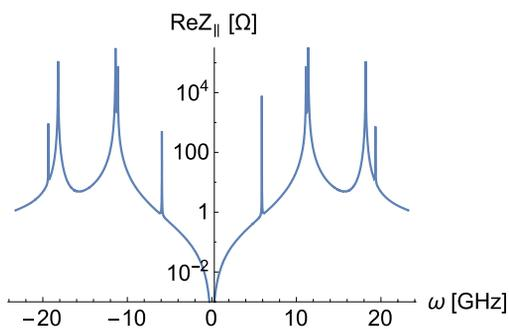
Figure 1:  $\text{Re}Z_{\parallel}(\omega)$  vs.  $\omega$  for HOMs in Table 1.
