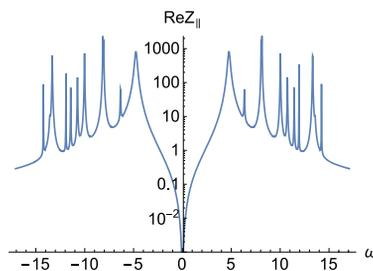
Figure 5:  $\text{Re}Z_{\parallel}(\omega)$  vs.  $\omega$  for HOMs in the PEP-II RF Cavities
