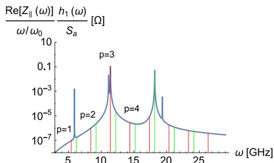
Figure 2: Summand of effective impedance for two different coupled-bunch modes (ion ring)
