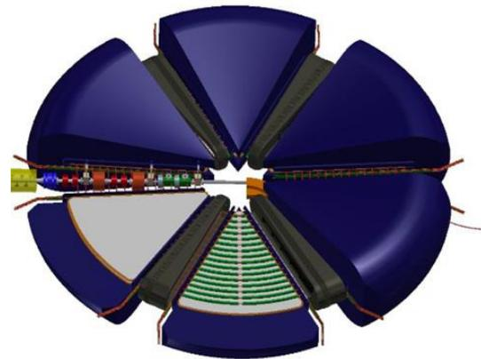
Figure 1: Cutaway view of a 100 MeV SFC, showing the 16-turn spiral trajectory, the superconducting slot cavities (dark grey), and the beam transport channels (green).
