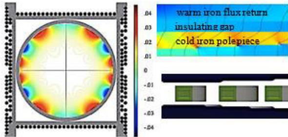
Figure 3: Left: Beam transport channel, showing detail of wire placement for quad and trim dipole windings; Upper right: cross-section of sector dipole, showing warm iron flux return, insulating gap, and cold iron pole plate; Lower right: positions of BTCs centered in each stair-step of the dipole aperture.
