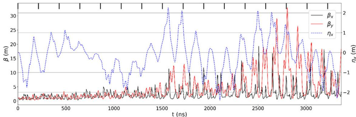
Figure 4: Lattice functions  $\beta_x, \beta_y, \eta_x$  for the entire SFC. The successive turns are indicated at the top.
