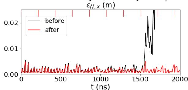
Figure 6: Evolution of the normalized horizontal emittance for roughly half of the SFC. Two cases are shown before and after optimization. Turn transitions are indicated at the top of the figure.
