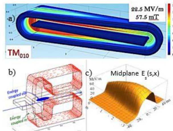
Figure 2: Superconducting cavity rf cavity, showing details of structure, location of couplers, midplane rf field.
