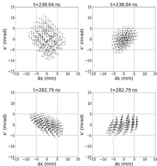
Figure 5: Poincaré sections from a single simulation of a bunch ( $N=14000$ ) illustrating emittance exchange between the horizontal (left) and longitudinal (right) spaces, via a synchro-betatron mechanism.
