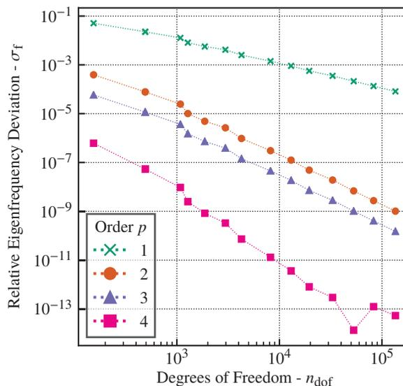
Figure 3: Eigenvalue deviation of the  $TM_{101}$ -Mode with respect to the analytical solution of a spherical cavity as a function of degrees of freedom for different geometry discretization orders.
