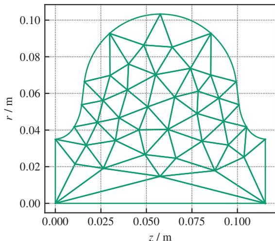
Figure 2: Finite elements of a TESLA-type mid-cell cavity triangulated with GMSH [7] using quadratic, i.e. second order, elements.
