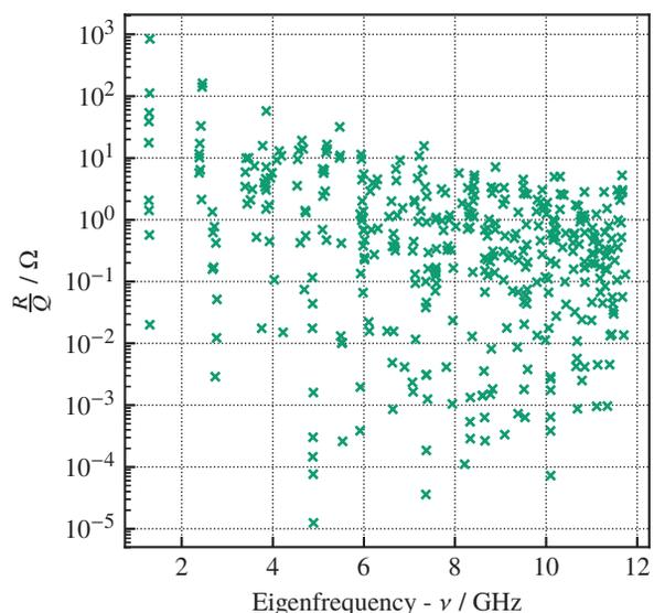
Figure 5: The longitudinal  $R/Q$  for the first  $n = 720$  monopole eigenvalues of the complete (9-cell) TESLA-type cavity structure.
