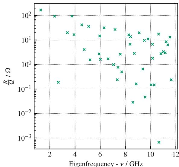
Figure 4: The longitudinal  $R/Q$  for the first  $n = 80$  monopole eigenvalues of a single TESLA-type mid-cell cavity.
