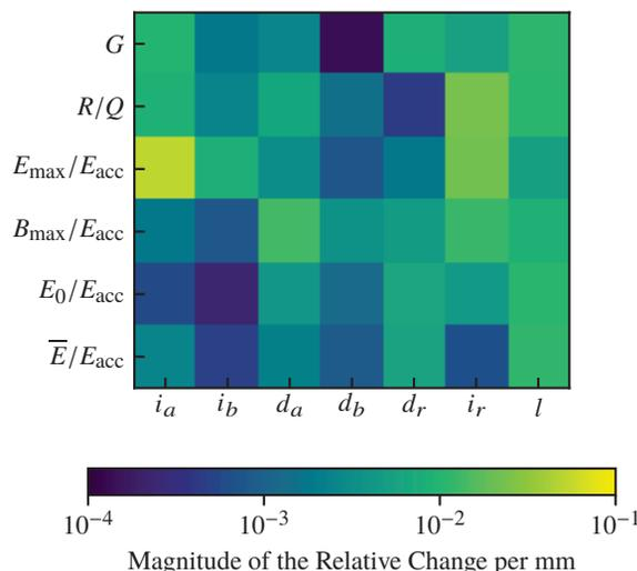
Figure 6: Jacobian of a TESLA-type mid-cell cavity with common figures of merit [11] as a function of the iris ellipse  $i_{a/b/r}$ , dome ellipse  $d_{a/b/r}$  geometry parameters as well as the length of the cell  $l$ , where  $a$  resp.  $b$  do represent the semi-resp. major-half axes of the ellipses and  $r$  the  $r$ -coordinate of the ellipses centroids.
