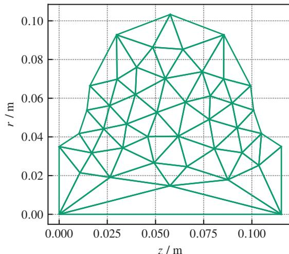
Figure 1: Finite elements of a TESLA-type mid-cell cavity triangulated with GMSH [7] using linear, i.e. first order, elements.
