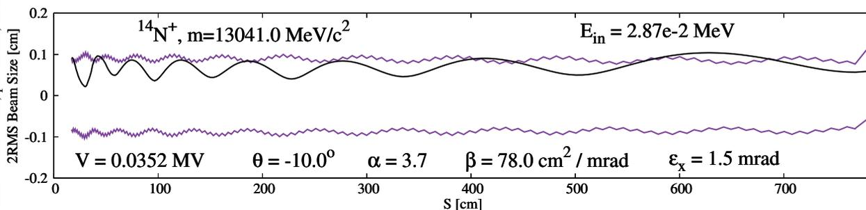
Figure 6: PARMTEQ simulation of an  $^{14}\text{N}^+$  beam, injected at 28.7 keV and accelerated to 2.142 MeV.  $V$  denotes the vane voltage,  $\theta$  the RF injection phase offset in 35.4 MHz degrees,  $\alpha$ ,  $\beta$  &  $\epsilon$  are the input Twiss parameters. The x & y envelope are the upper and lower purple curves, while the longitudinal envelope, divided by 10, is in black.
