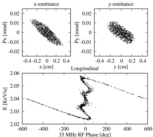
Figure 2: PARMELA simulated  $A/q = 30$  beam using 3000 particles, time focussed at the RFQ entrance, 5 m downstream from the prebuncher.
