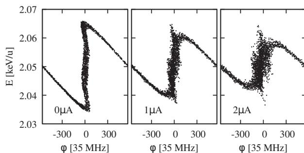
Figure 4: PARMELA simulated  $A/q = 30$  beam using 2000 particles, showing the effects of space charge at the entrance of the RFQ at different averaged beam currents.
