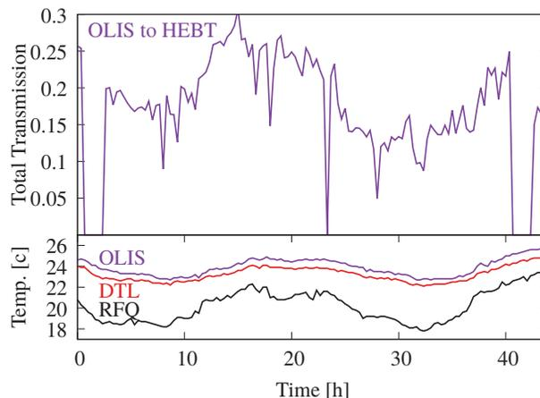
Figure 1: Top:  $^{20}\text{Ne}$  transmission readings from the off-line ion source (OLIS), each 20 minutes for 44 hours. Faraday cup readings have been normalized to the cup immediately upstream, showing beam transmission between 0 and 1 for the labeled sections. Gaps in data caused by RF trips. Bottom: ISAC-I experimental hall ambient air temperature, sampled at identical time intervals.
