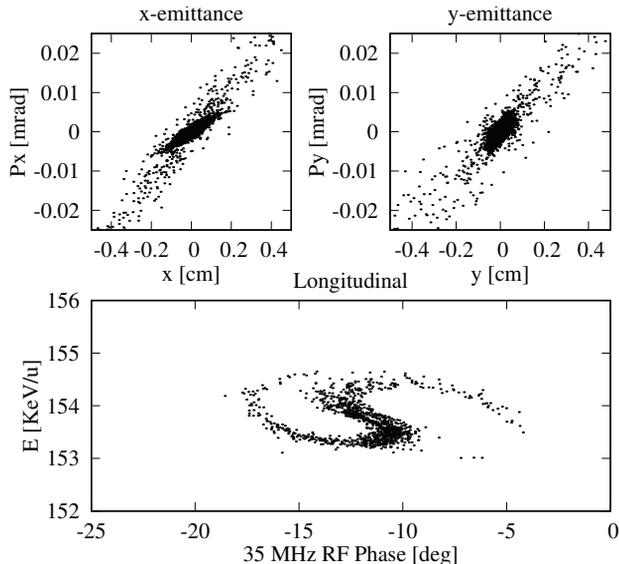
Figure 5: PARMTEQ simulated  $A/q = 30$  beam using 3000 particles, accelerated through ISAC RFQ.
