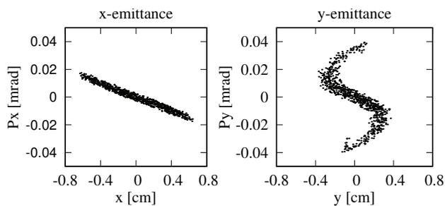
Figure 3: PARMELA simulated  $A/q = 30$  beam using 3000 particles, mismatched at the RFQ entrance and showing effects of aberration, 5 m downstream from the prebuncher.
