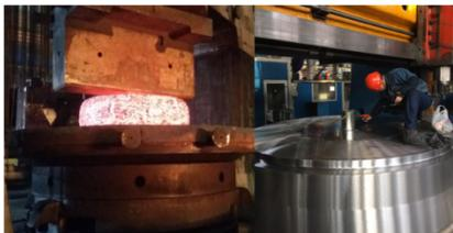
Figure 7: The pure iron forging pieces for the main magnet of CYCIAE-250.
