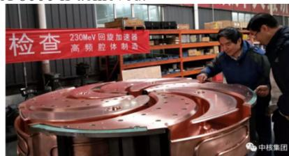
Figure 8: RF cavities of CYCIAE-230.
