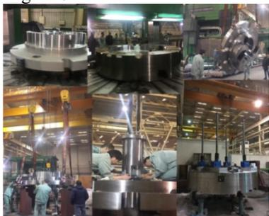
Figure 5: Highlights of main magnet fabrication. (From left to right, top to bottom: fine machining of pole and yoke, turnover of pole pieces, fine alignment of pole, installation of central plug and lifting system).
