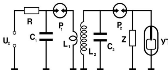
Figure 2: Accelerating tube triggering circuit: R – charging resistance; C<sub>1</sub> – tank capacitor; P<sub>1</sub> – primary circuit discharger; L<sub>1,2</sub> – Tesla coil primary and secondary winding inductance; C<sub>2</sub> – Tesla coil secondary circuit capacitance; P<sub>2</sub> – discharger; Z – reactance.
