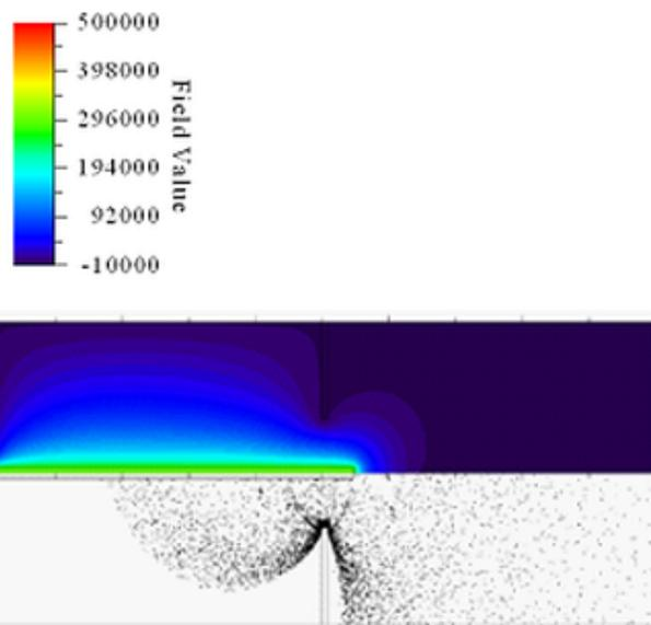
Figure 5: Field potential (upper part) and electrons (lower part of each picture) distribution in accelerating tube.
