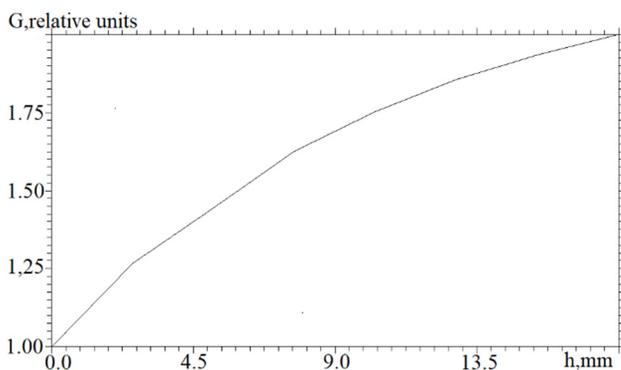
Figure 7: Dose rate of generated radiation G on distance from the front end of a cathode disk to the front end of an anode.
