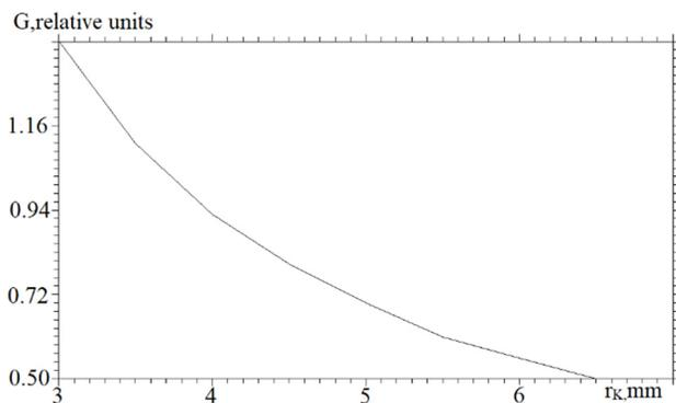
Figure 6: Dose rate of generated radiation G on cathode radius  $r_K$ .
