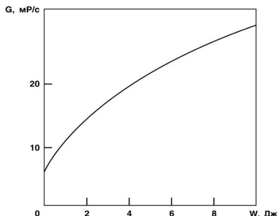
Figure 4: The measurement results of the dose rate of generated radiation  $G$  on power  $W$  stored in the tank capacitor.
