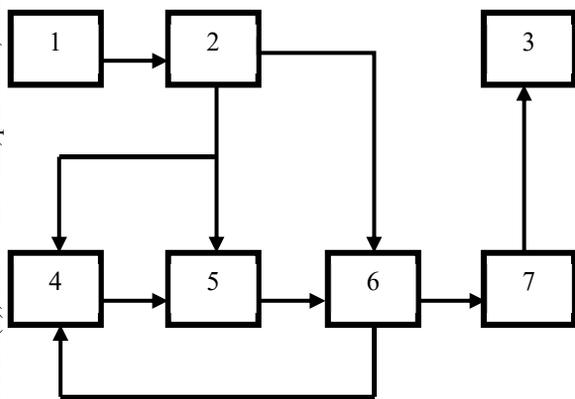
Figure 3: The block diagram of x-ray quants generator. 1- supply-line filter, 2- power supply unit, 3- high voltage unit, 4- control unit, 5- pulse generator, 6- power amplifier, 7-voltage multiplier.
