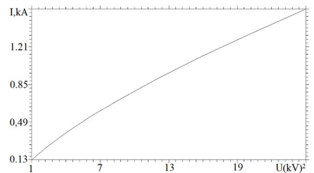
Figure 8: Anode current dependence on square of accelerating field.
