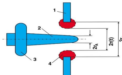
Figure 1: Accelerating tube electrodes for X-ray generation. 1 – cathode, 2 – anode, 3 – protective screen from cathode sputtering, 4 – plasma cloud.
