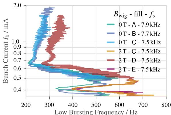
Figure 3: Low bursting frequency (periodicity of radiation outbursts) as a function of bunch current for different fills. Shift in frequency visible for CLIC<sub>DW</sub> at 0 T or 2 T.
