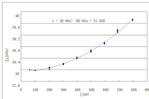
Figure 1: Variation of the synchrotron oscillation tune with beam current for BER (“♦”: measurement data, solid line: fitting curve).
