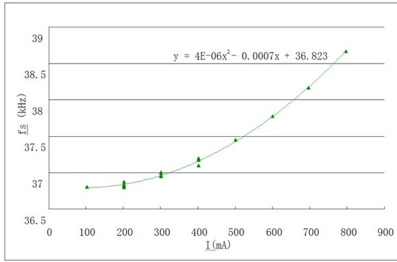
Figure 2: Variation of the synchrotron oscillation tune with beam current for BPR (“▲”: the measurement data, solid line: fitting curve).
