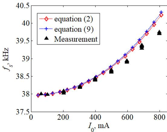
Figure 3: Theoretical estimation on the coherent synchrotron oscillation frequency versus beam current, and compared with the measured data (BER).
