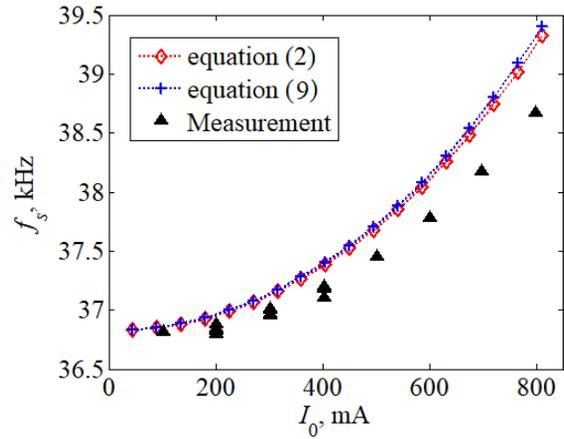
Figure 4: Theoretical estimation on the coherent synchrotron oscillation frequency versus beam current, and compared with the measured data (BPR).
