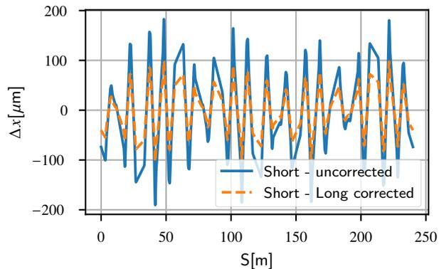
Figure 6: Orbit distortions for short bunches in the PPMM case before (blue) and after (orange) correction, where a correction for long bunches was applied.
