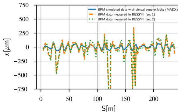
Figure 8: Comparison between simulated orbit distortion using the virtual kickers (blue) and measured orbits in the machine using the two sets of orbit correctors from Table 2 (orange and green respectively).
