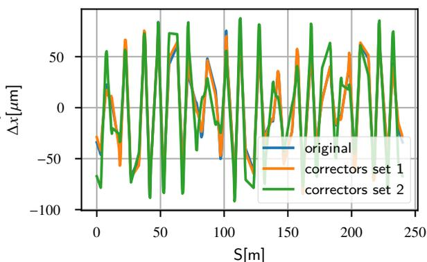
Figure 7: Orbit distortions for the PPMM case using the virtual kickers (blue), set 1 of correctors from Table 2 (orange) and set 2 of correctors from Table 2 (green).
