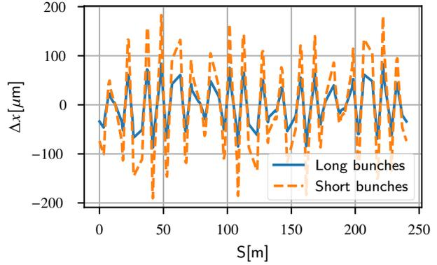
Figure 4: Orbit distortions for long (blue) and short (orange) bunches in the PPMM case.
