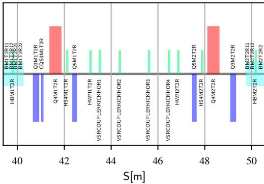
Figure 3: Lattice elements in the region where the new cavities will be installed, notice the presence of the four virtual horizontal kickers used to simulate the FPC kicks (VSRCOUPLERKICKHOR).
