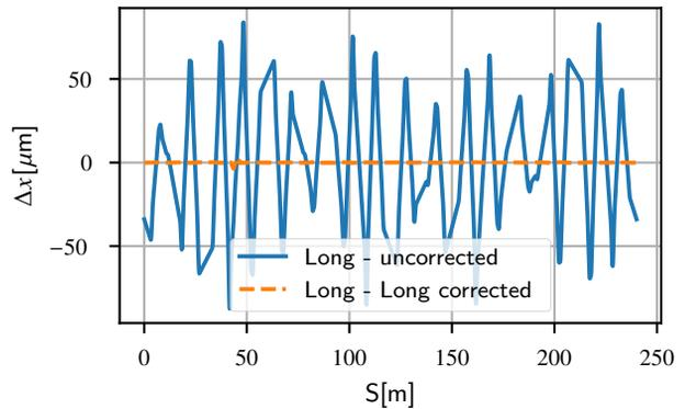
Figure 5: Orbit distortions for long bunches in the PPMM case before (blue) and after (orange) correction, where a correction for long bunches was applied.
