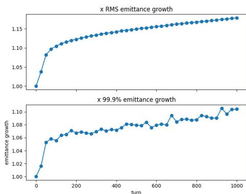
Figure 3: RMS and 99.9% emittance growth during the first 1000 turns of the perfectly periodic lattice with initial space charge tune shift of about 0.9 with no electron lenses.
