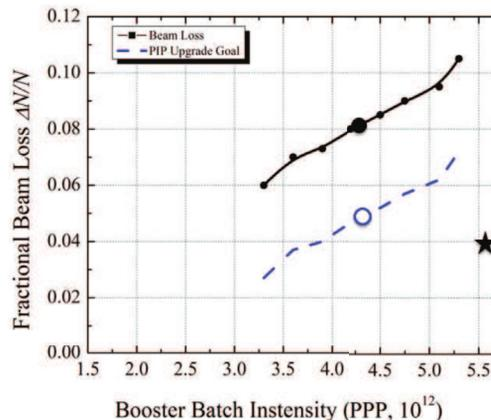
Figure 1: Fractional beam losses in Fermilab's 8 GeV proton Booster synchrotron vs. the total intensity of the batch of 84 bunches in the accelerator. The dashed blue curve shows the level at the recently reached 700 kW level while the star shows the anticipated level at the end of the PIP-I+ upgrade.
