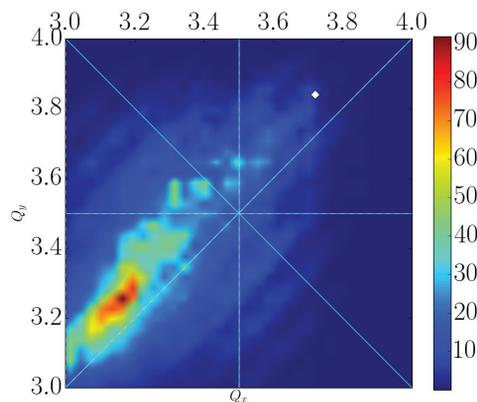
Figure 5: Tune power density in the first 200 turns of the perfectly periodic lattice. Each point on the plot represents the tune power spectrum present in all the particles. The diamond at (3.72,3.84) is the bare lattice tune without space charge. The faint lines parallel to the diagonal separated from the main population by twice the synchrotron tune are caused by the modulation of space charge by synchrotron motion.
