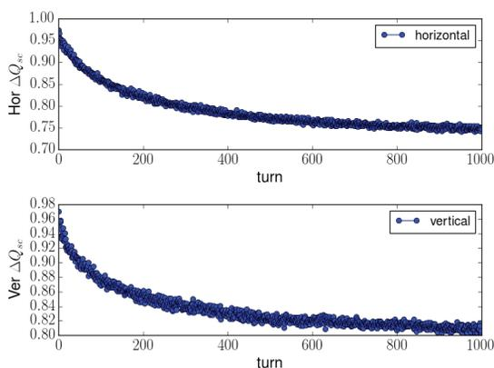
Figure 4: Evolution of the space charge tune shift during the first 1000 turns of the perfectly periodic lattice.
