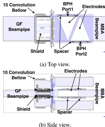
Figure 1: 3D Geometry of BPH in CST MWS.
