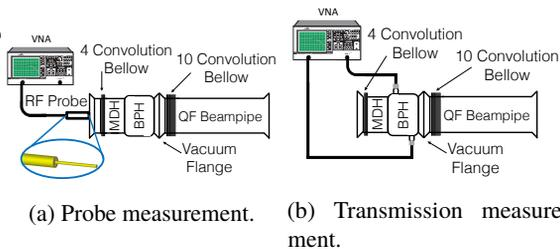
Figure 2: Test measurement setup in the laboratory.
