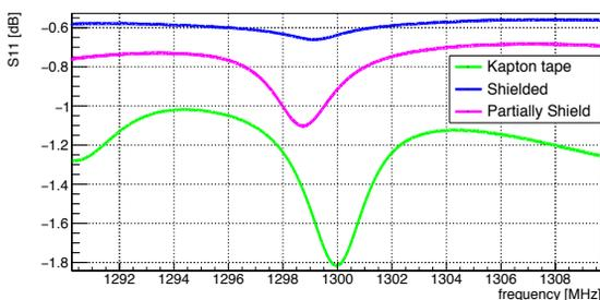
Figure 3: Probe measurements at 1.3 GHz for the cases of unshielded, shielded and partially shielded flanges shown in green, blue and pink respectively.
